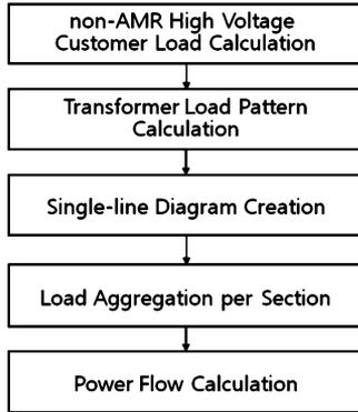
Fig. 2. Load calculation process.
