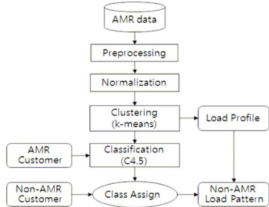
Fig. 3. Calculation process for the load pattern of the non-AMR high-voltage customer.
