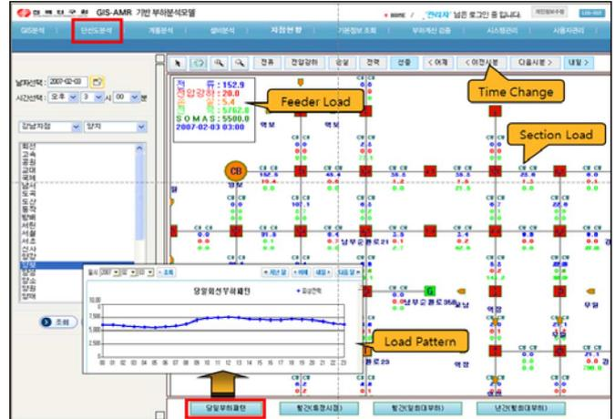
Fig. 5. Load analysis using the SLD.
