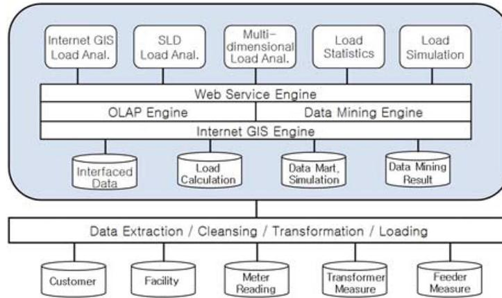
Fig. 1. Structure of the spatiotemporal load-analysis model.
