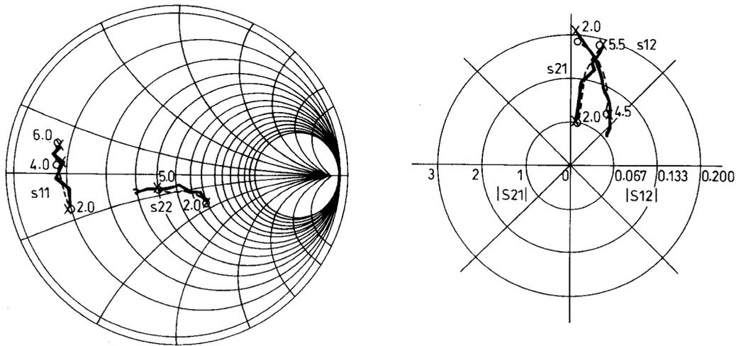
**Fig. 8** *S*-parameter–frequency variations for  $V_{CE} = 8V$ ,  $I_C = 30mA$  at common emitter configuration of transistor NE219
