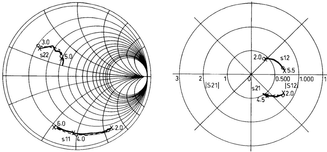
**Fig. 7** *S*-parameter–frequency variations for  $V_{CE} = 8.0V$ ,  $I_C = 10mA$  at the common collector configuration of transistor NE219
