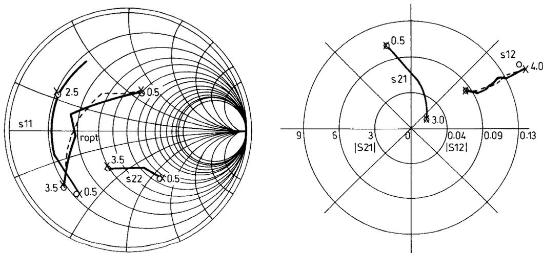
**Fig. 9** *S*- and *N*-parameter–frequency variation for  $V_{CE} = 10V$ ,  $I_C = 5mA$  at the common emitter configuration of transistor NE02135 (SFG)
