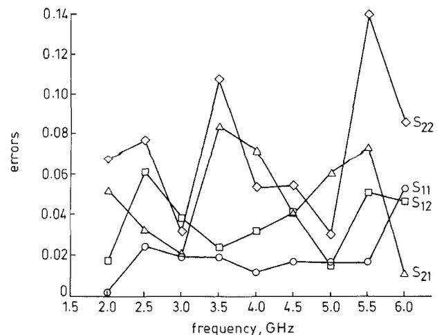
**Fig. 6** Error-frequency distributions for  $V_{CE} = 8\text{V}$ ,  $I_C = 20\text{mA}$  at the common collector configuration of the transistor NE219 (WFBG)
