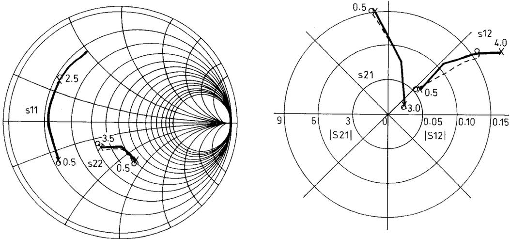
**Fig. 11** S-parameter-frequency variations for  $V_{CE} = 10V$ ,  $I_C = 10mA$  at the common emitter configuration of transistor NE02135 (WFBG)
