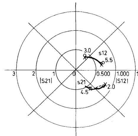
Fig.5 S-parameter-frequency variations for  $V_{CE} = 8V$ ,  $I_C = 20mA$  at the common collector configuration of the transistor NE219 (WFBG).  $E_{11} = 0.019730$ ,  $E_{21} = 0.035988$ ,  $E_{12} = 0.049394$ ,  $E_{22} = 0.071714$ ,  $E_i = 0.044207$
