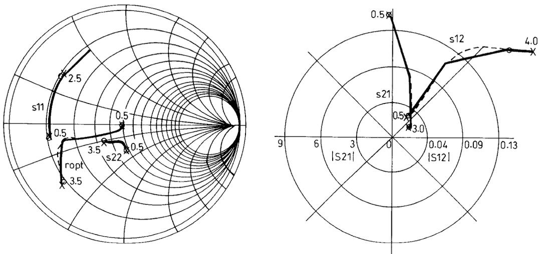
**Fig. 12** S-parameter-frequency variations for  $V_{CE} = 10V$ ,  $I_C = 30mA$  at the common emitter configuration of transistor NE02135 (SFG)
