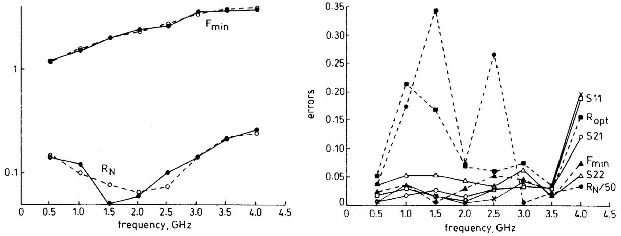
**Fig. 10** Error-frequency distributions for  $V_{CE} = 10V$ ,  $I_C = 5mA$  at the common emitter configuration of transistor NE02135 (SFG)
