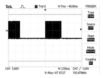
When the third port on the "industry standard architecture" adapter was opened at 115.2K bps, the data rate on the first serial port dropped to only 33K bps.
