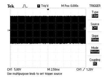
With one port on the "industry average architecture" adapter open at the standard baud rate of 115.2K bps, data was transmitted in bursts rather than in a continuous stream and the actual data rate was only approximately 65K bps.
