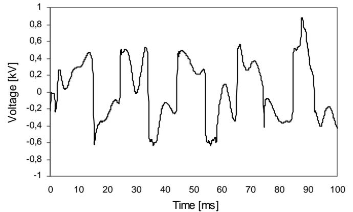
Figure 5. Voltage waveform at the Arc Furnace (Bus 7)
