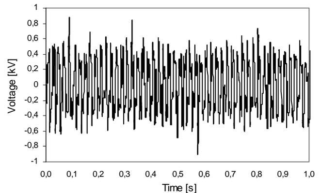
Figure 8. Voltage waveform at the Arc Furnace (Bus 7)
