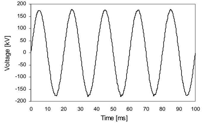
Figure 3. Voltage waveform at the PCC (Bus 2)
