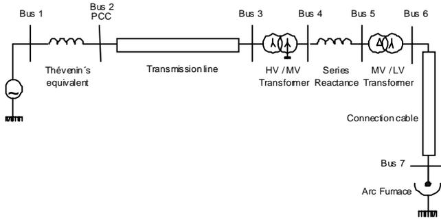
Figure 2. Electrical network supplying the arc furnace
