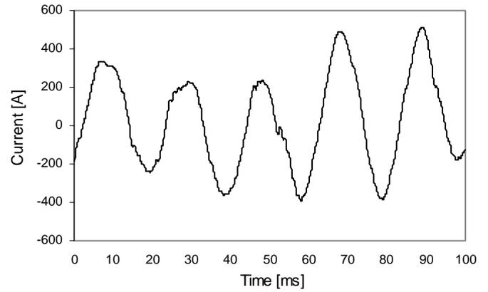
Figure 4. Current waveform at the PCC (Bus 2)
