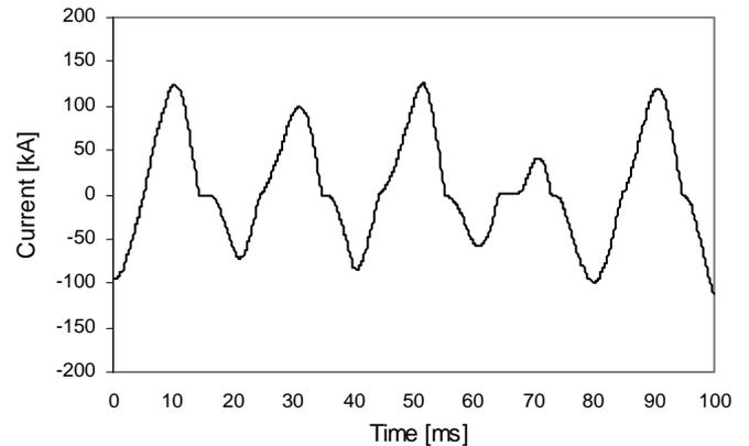
Figure 6. Current waveform at the Arc Furnace (Bus 7)
