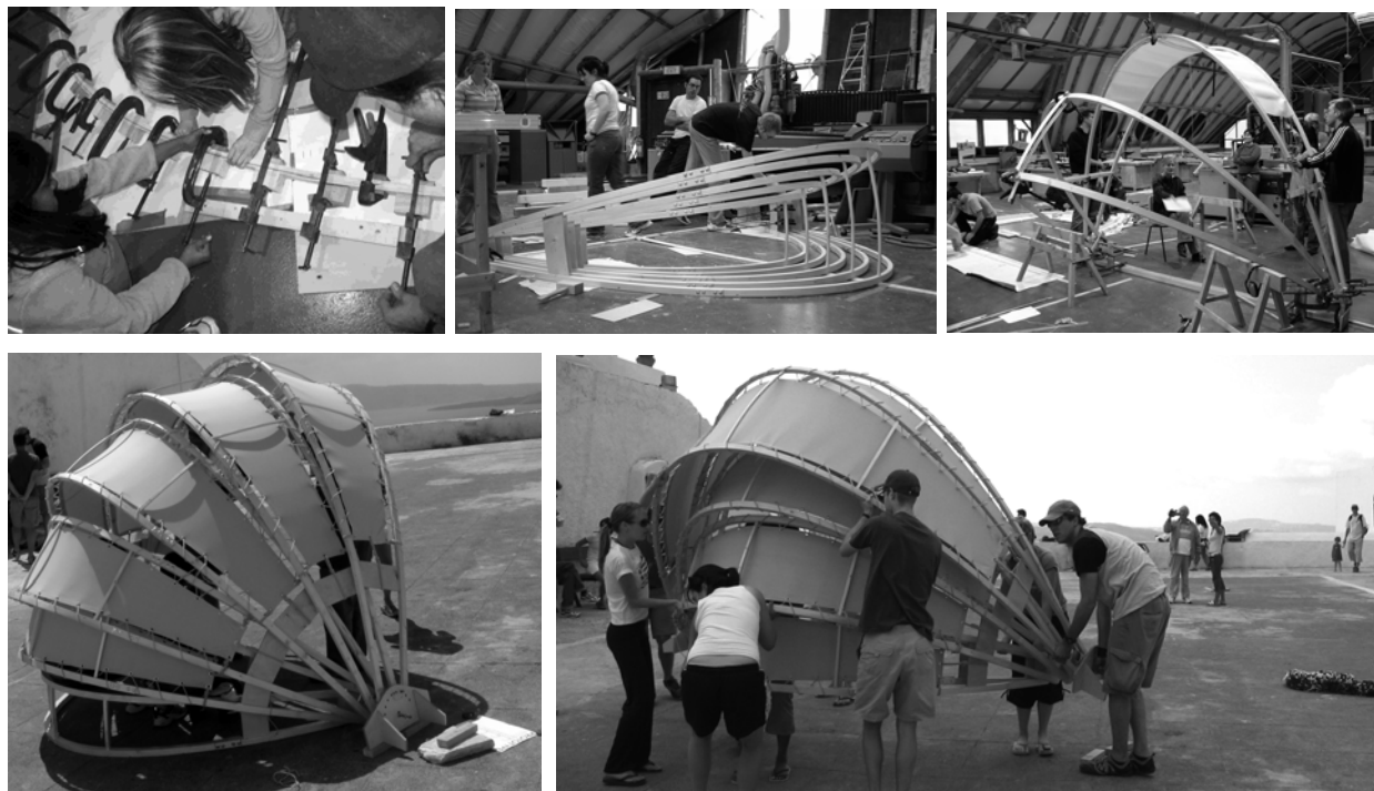
Figure 9: Making and assembling the heliotropic bench at AA School's Hooke Park laboratories and on location in Oia, Santorini.
