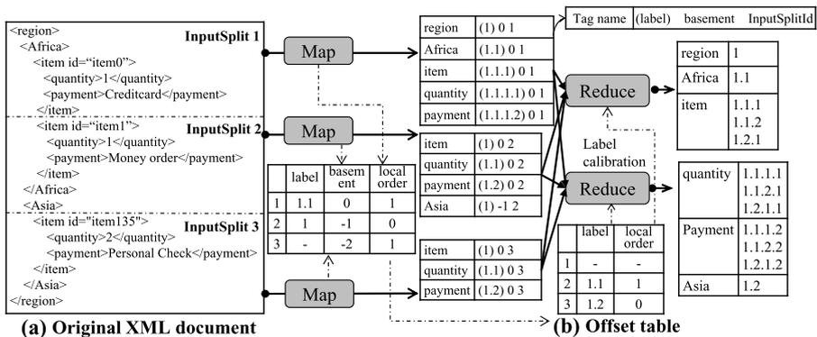
Fig. 5 An illustration of parallel prefix-based labeling
