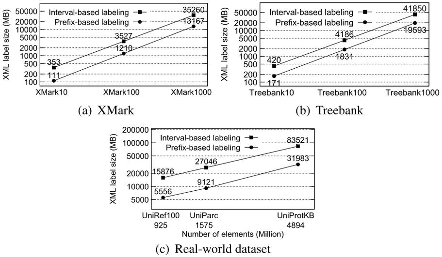
Fig. 9 The size of XML labels
