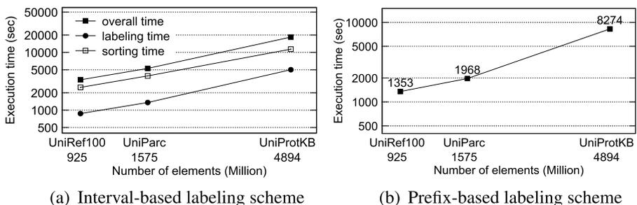
**Fig. 1** Execution time for sequential XML labeling algorithms
