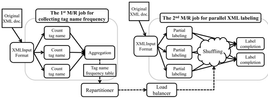
**Fig. 6** Overview of the optimized version of parallel labeling process
