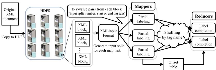
Fig. 3 Overview of parallel XML labeling with MapReduce
