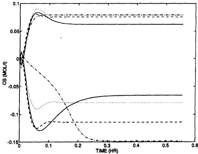
Fig. 12. Asymmetric Model response for  $\pm 6$  (mol/l) step changes in input. Actual reactor (solid), linear (dotted), 3 neuron RDNN (dashed).
