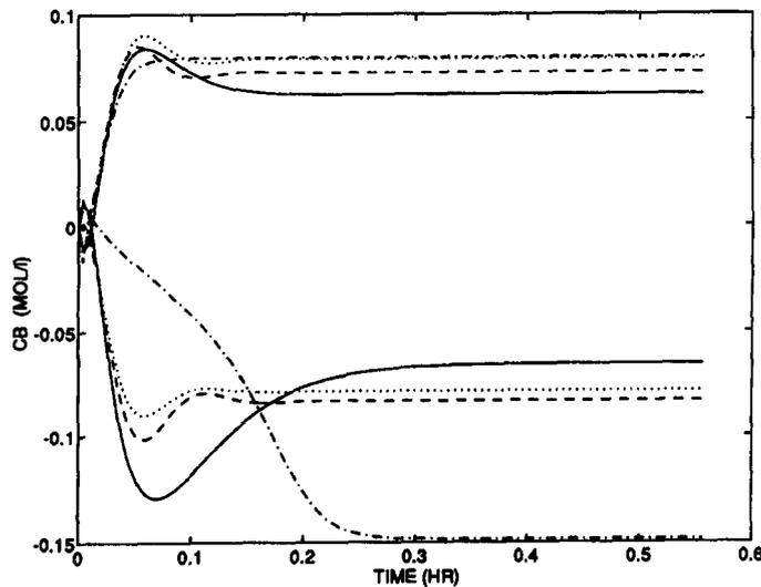
Fig. 10. Model comparison for  $\pm 6$  (mol/l) step changes in input. Actual reactor (solid), linear (dotted), FANN (dash-dot), 2 neuron RDNN (dashed).
