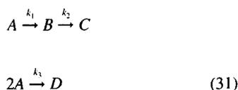
For constant density and ideal reactor residence time, the balance equations for the concentrations of cyclopentadiene,  $c_A$ , and cyclopentanol,  $c_B$ , are:
