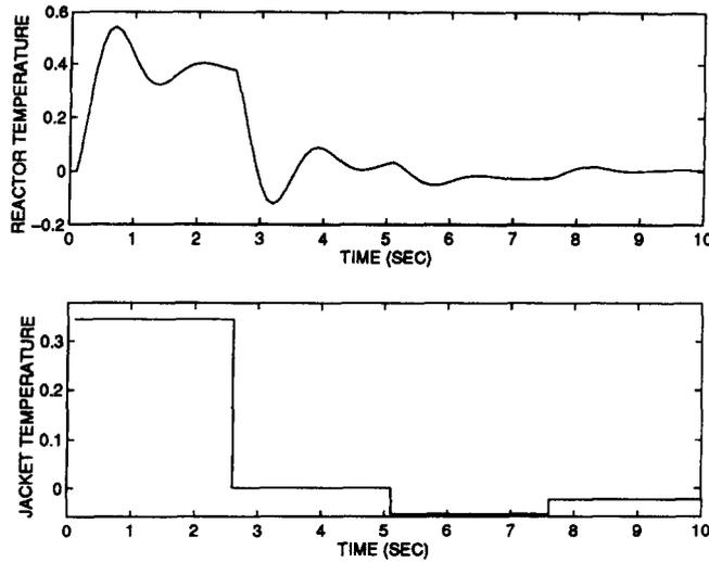
Fig. 3. Input/output data for linear identification.
