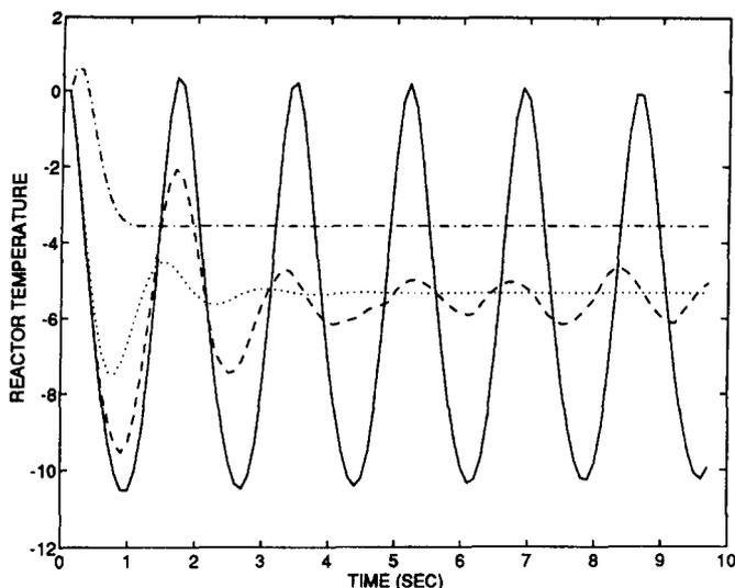
Fig. 7. Model comparison for  $-5$  step change in input. Actual reactor (solid), linear (dotted), FANN (dash-dot), RDNN (dashed).
