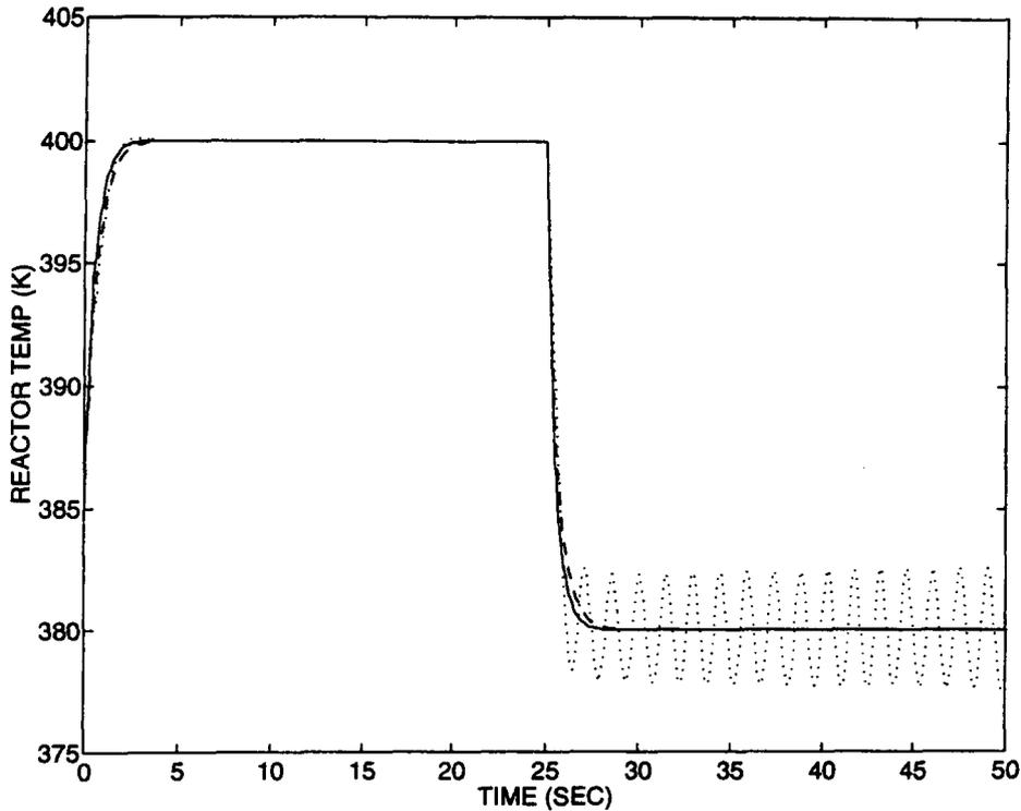
Fig. 14. Closed-loop setpoint response. Reference trajectory (solid), RDNN controller (dotted), linear controller (dashed).
