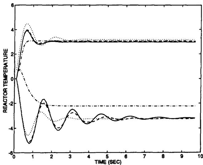
Fig. 6. Model comparison for  $\pm 3$  step changes in input. Actual reactor (solid), linear (dotted), FANN (dash-dot), RDNN (dashed).
