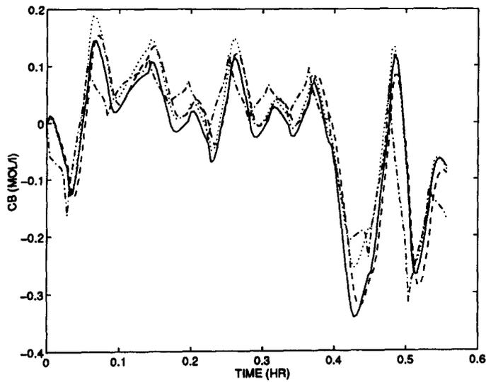
Fig. 9. Model comparison for random input sequence. Actual reactor (solid), linear (dotted), FANN (dash-dot), 2 neuron RDNN (dashed).
