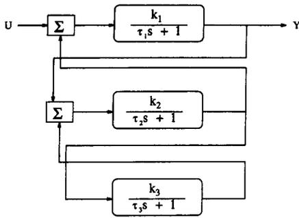
Fig. 2. Generalized 3 neuron structure for dynamic neural network.
