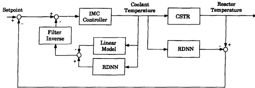
Fig. 13. Closed-loop control structure.
