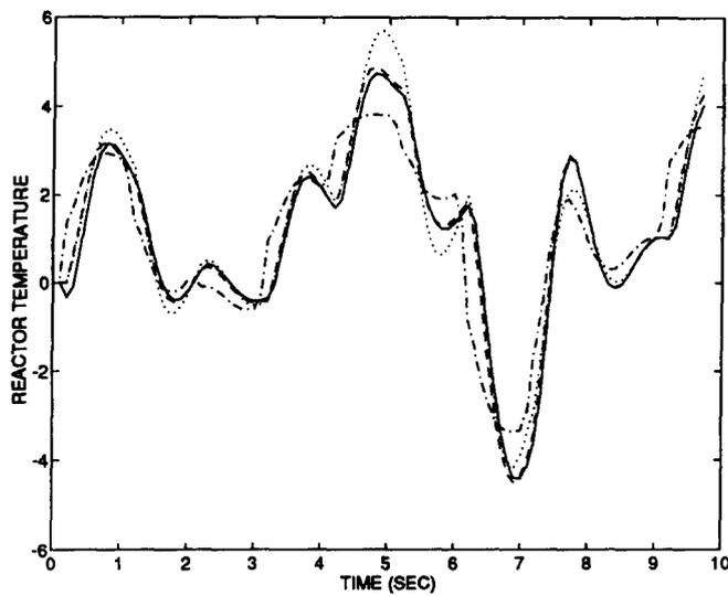
Fig. 5. Model comparison for random input sequence. Actual reactor (solid), linear (dotted), FANN (dash-dot), RDNN (dashed).
