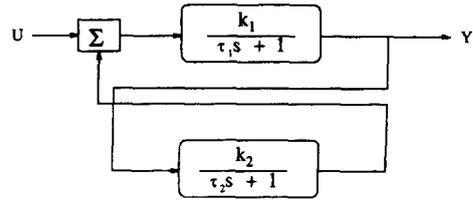
Fig. 1. Dynamic recurrent network model.
