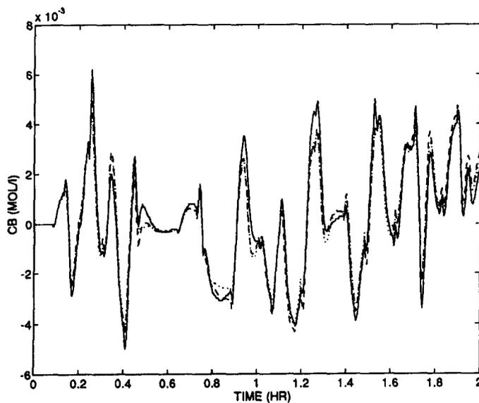
Fig. 8. Comparison of second and third order linear models to small input perturbations. Actual (solid), second order (dotted), third order (dashed).
