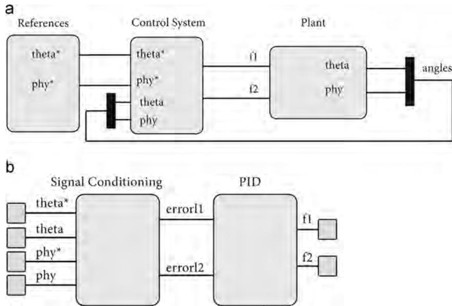
Fig. 4. A scheme of the controlled hydraulic prosthesis system (a) and of the control system block configuration with the errors and duty cycle signals (b).
