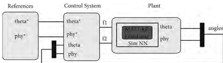
Fig. 5. A scheme of the controlled hydraulic prosthesis system with the ANN block integrated into the system plant.
