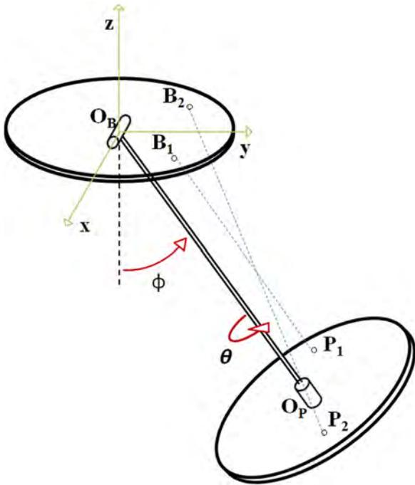
Fig. 2. The 3D kinematics scheme of the parallel mechanism of the actuated hydraulic prosthesis.
