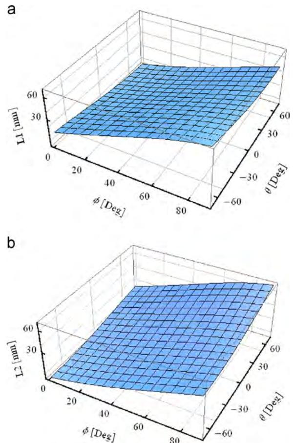
Fig. 3. The nonlinear relations between the two front cylinders rods elongations (left (a) and right (b)) and the forearm rotations of the hydraulic prosthetic device.
