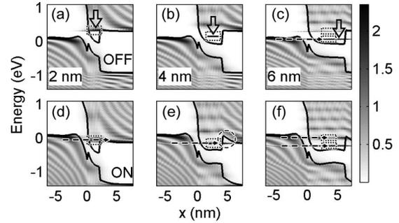
Fig. 3. (a)–(c) LDOS of the HJ TFETs for different  $L_{HJ} = 2, 4,$  and  $6$  nm at the OFF-state ( $V'_{GS} = 0$  V), with quantum states highlighted within the dotted boxes in the well structure. (d)–(f) LDOS of the corresponding devices at the ON-state ( $V'_{GS} = 0.6$  V), and the dash arrows indicate where BTB tunneling occurs. The colorbar indicates the LDOS values with a unit of  $[\times 10^{23} \text{ cm}^{-2} \cdot \text{eV}^{-1}]$  and is applied to all plots.
