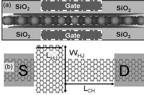
Fig. 1. (a) Side-view schematic of a simulated GNR TFET and (b) atomic model of the HJ TFET. The dark gray zones in (b) represent the source and the drain regions, and  $L_{HJ}$  and  $W_{HJ}$  are the length and width for the HJ region, respectively, whereas  $L_{CH}$  is the channel length. The gate length,  $L_G = L_{HJ} + L_{CH}$  when the gate is fully covering the HJ region, i.e.,  $GC = 1$ .
