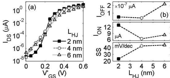
Fig. 2. (a) Transfer characteristics of GNR HJ TFETs with different HJ lengths.  $L_{HJ} = 2, 4,$  and  $6$  nm, respectively, where  $V'_{GS} = V_{GS} - V_{DS}/2$  [19]. The applied drain bias ( $V_{DS}$ ) is  $0.6$  V. (b) Extracted OFF-state current ( $I_{OFF}$ ), ON-state current ( $I_{ON}$ ), and SS versus  $L_{HJ}$ . The dash lines are line guides.
