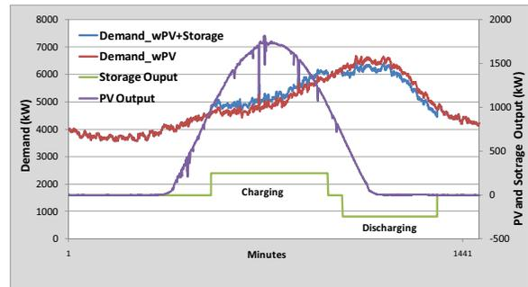
**Fig. 4. Using storage to shift PV generation**
