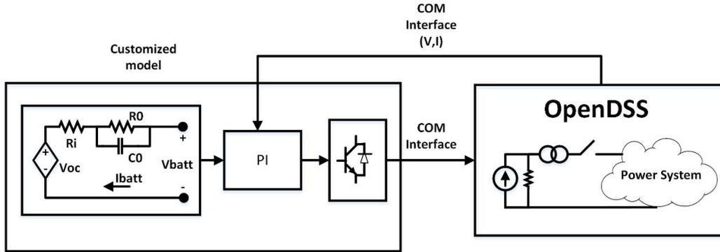
Fig. 7. Proposed simulation including a customized model
