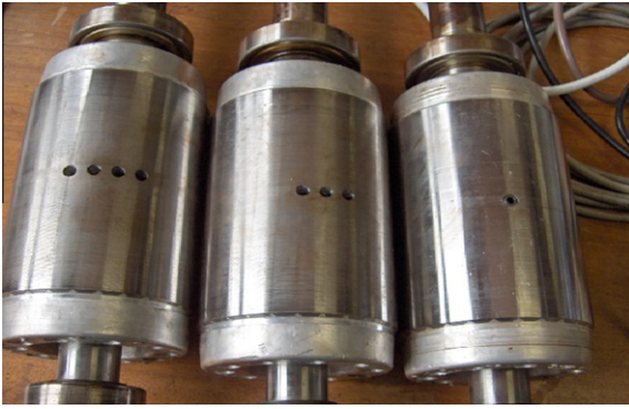
Fig. 2. Broken rotor bars.
