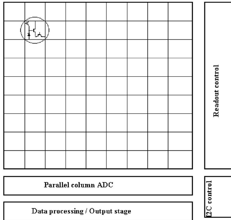
Fig. 3. Architecture of a CMOS sensor. The pixels are read in column and the data are digitised in parallel. On the periphery, other blocks can be integrated for the control of the circuits and for the data processing.
