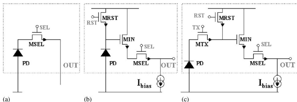
Fig. 1. The dashed line indicates the pixel area: (a) Schematic of a Passive Pixel Sensor (PPS). (b) Baseline, 3-MOS Active Pixel Sensor (APS). (c) 4-MOS APS with transfer gate (MTX).
