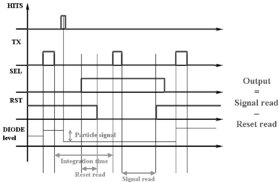
Fig. 4. Timing diagram of the 4-MOS pixel with transfer gate.
