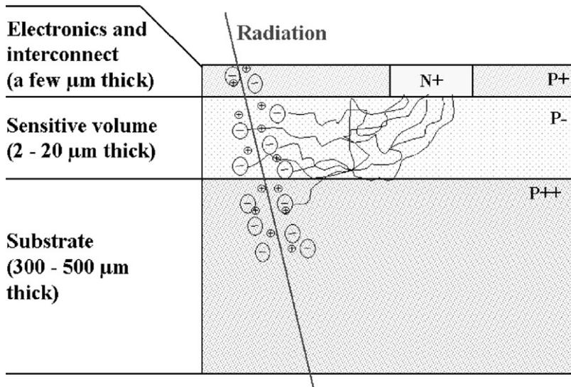
Fig. 2. Cross-section of a CMOS process showing the functioning of the proposed 100% fill factor structure.
