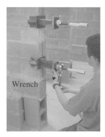
Fig. 4—Manually stressing a GFRP bar with a wrench
