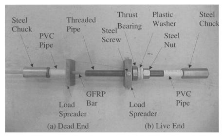
Fig. 1-Hand-held device components
