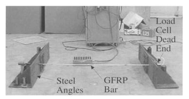
Fig. 6—Test setup for component evaluation
