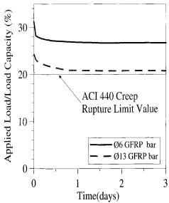
Fig. 7—Load relaxation of GFRP bars
