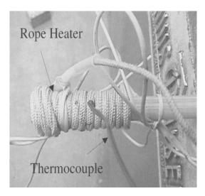
Fig. 2—Heating of a GFRP bar
