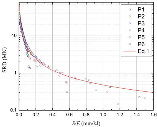
Fig. 7. Soil resistance versus  $S/E$ .
