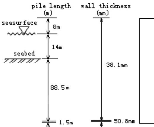
Fig. 3. Pile calculation model for wave equation analysis.
