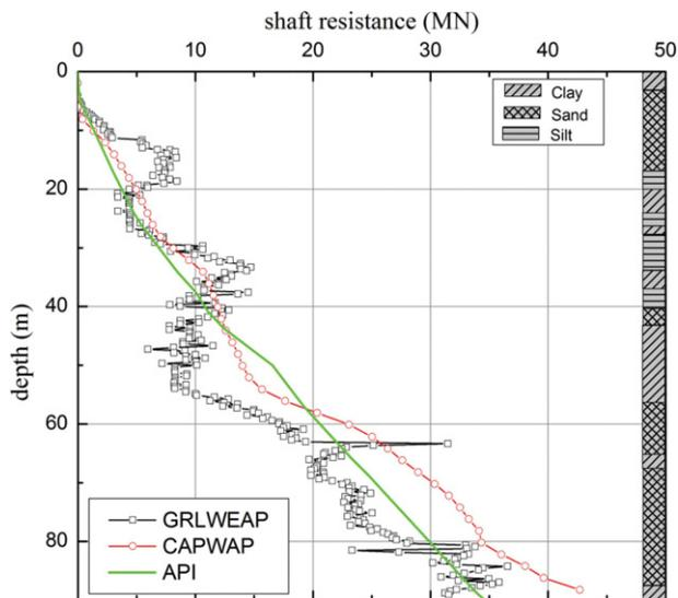
Fig. 9. Shaft friction along the pile.
