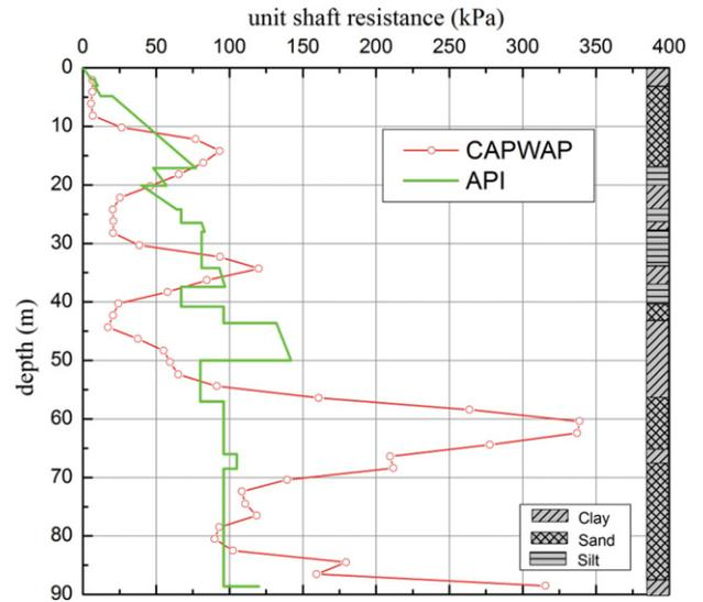
Fig. 10. Unit shaft resistance.
