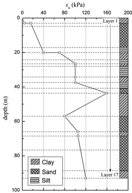
Fig. 1. Soil undrained shear strength.
