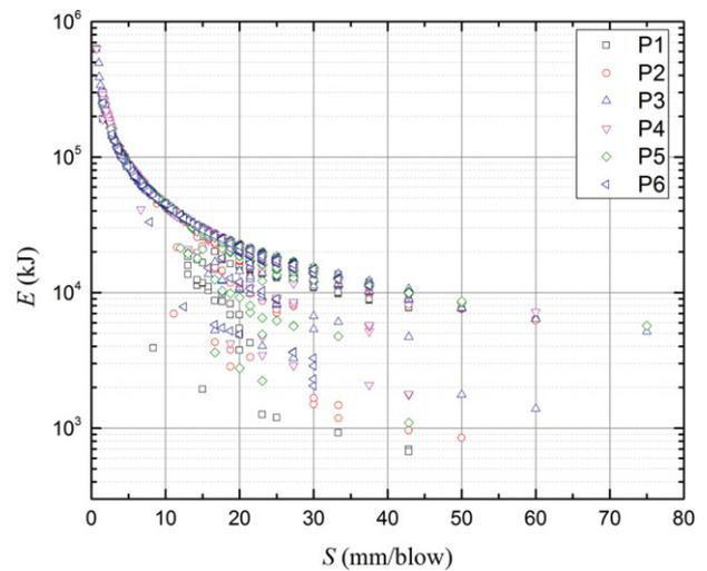
Fig. 6. Blow energy versus settlement.
