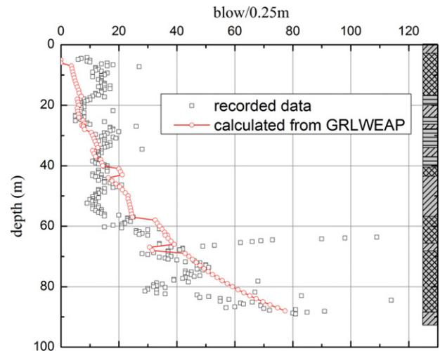
Fig. 4. Blowcount versus depth.
