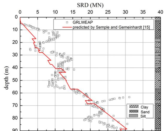
Fig. 5. Soil resistance to driving versus depth.
