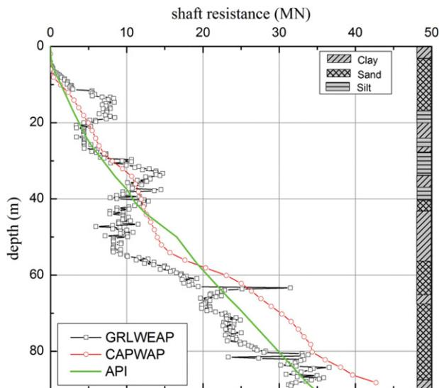
Fig. 9. Shaft friction along the pile.
