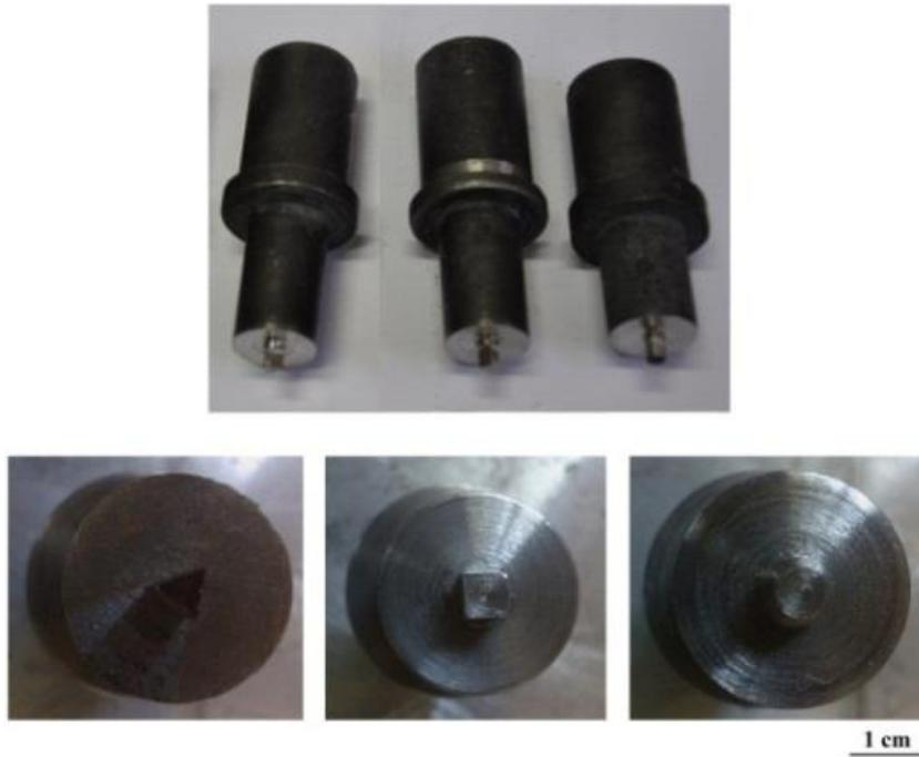
Fig. 1. FSW tool pin profiles.
