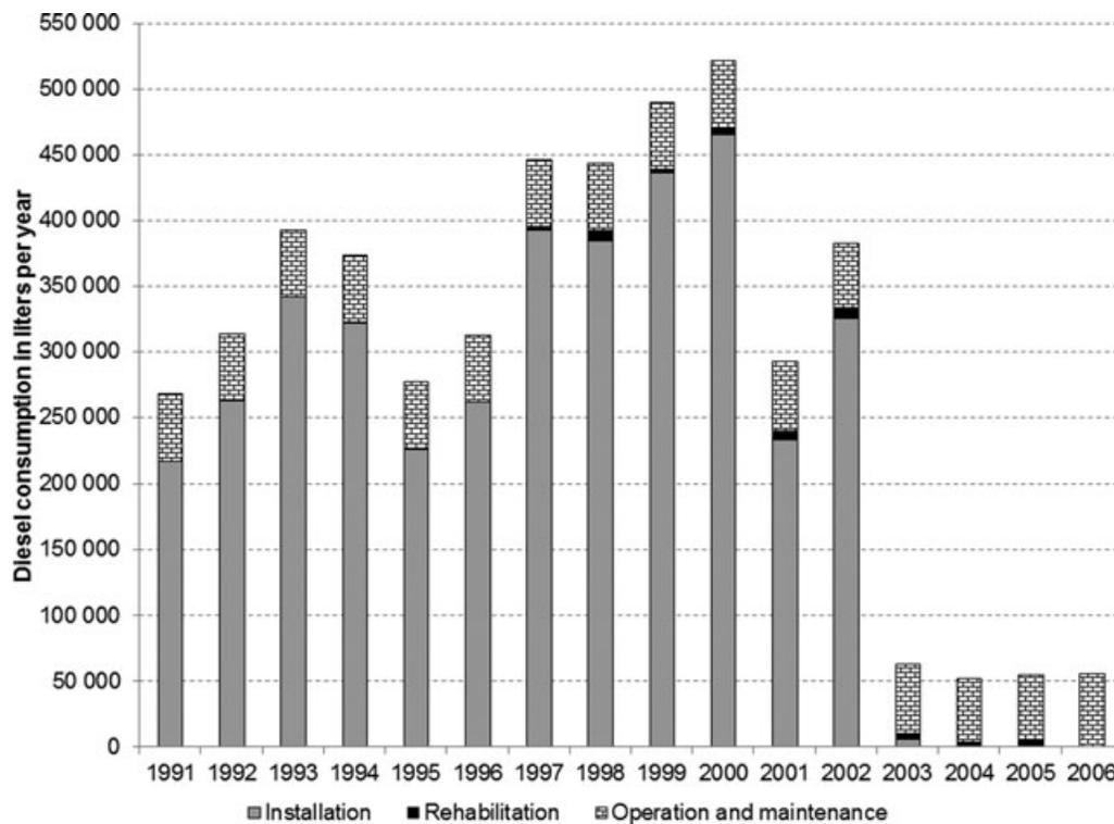
**Figure 6** Diesel fuel consumption in different life cycle phases of the water pipeline network, 1991–2006.
