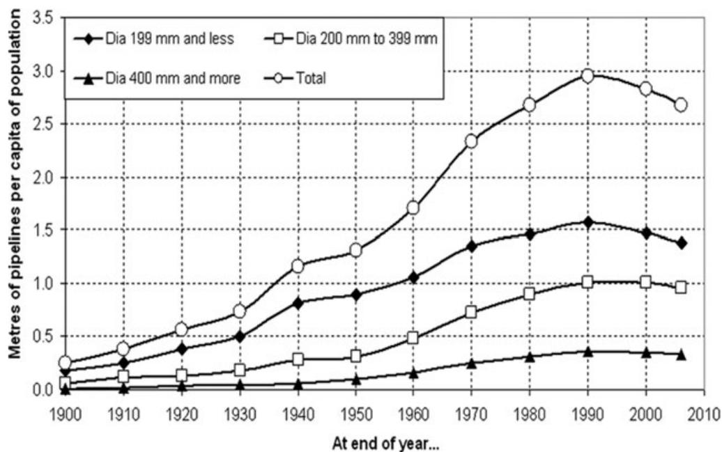
**Figure 3** Meters per capita over time of functioning water pipelines in Oslo.
