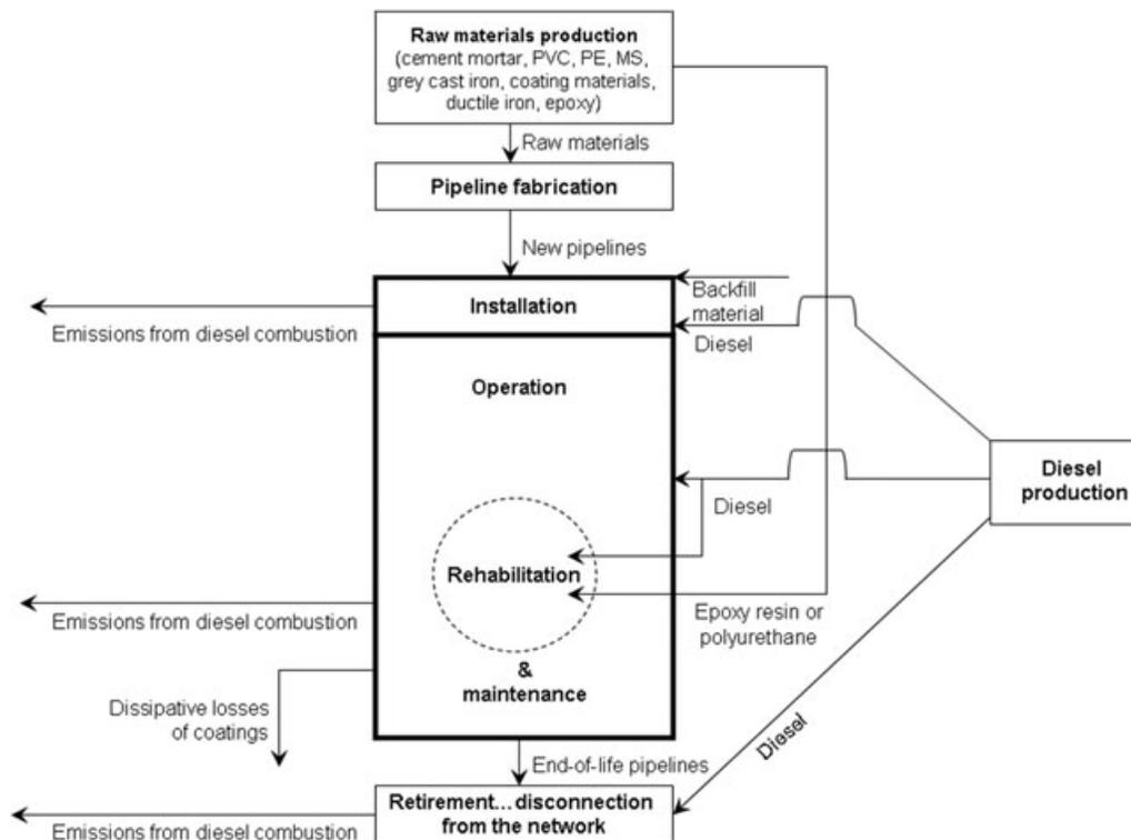
**Figure 2** Material and energy flows in the water pipeline network. PVC = polyvinyl chloride; PE = polyethylene; MS = mild steel.
