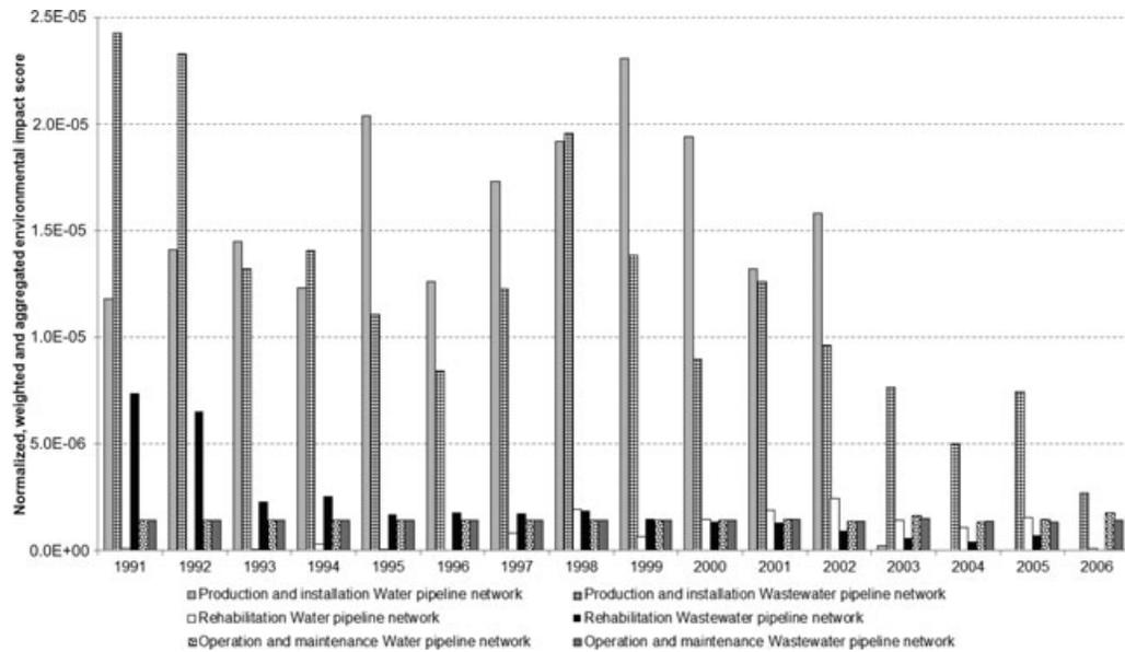
**Figure 7** Annual environmental impact from Oslo’s water and wastewater pipeline networks—contribution of each phase of the life cycle.
