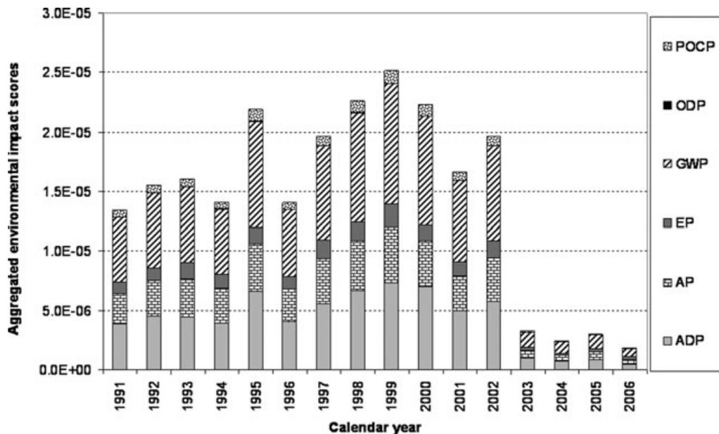
**Figure 8** Annual environmental impact from Oslo’s water pipeline network—contribution of different types of environmental impact (refer to the subsection “Determining environmental (LCA) impacts” for the expansions of the acronyms in the legend).
