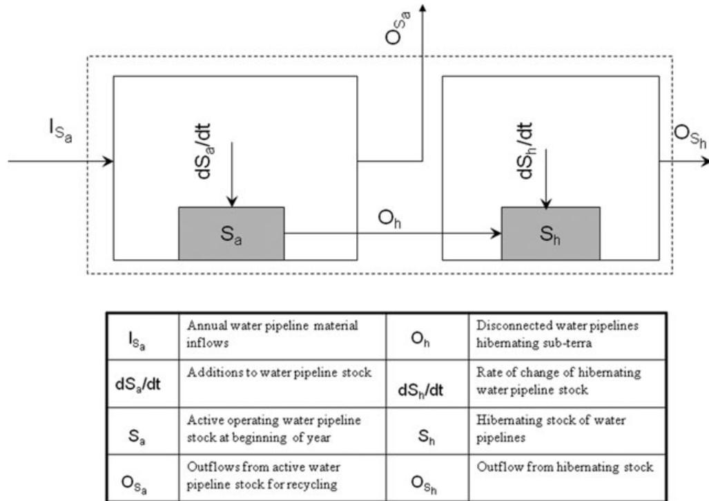
**Figure 1** Understanding pipeline material flows from a dynamic material flows analysis (MFA) perspective (dotted lines in the figure indicate the system boundaries).
