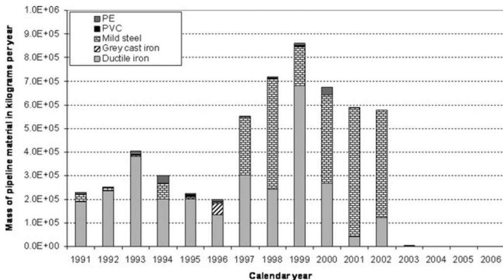
**Figure 5** Annual pipeline material inflows to the water pipeline network, 1991–2006.
