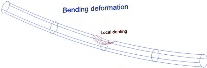
Fig. 1. Tube deformation under lateral transverse loading.
