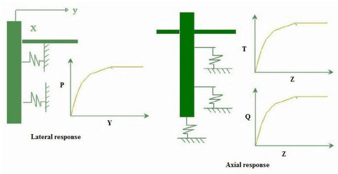
Fig. 1. Pile soil interaction stiffness curves.
