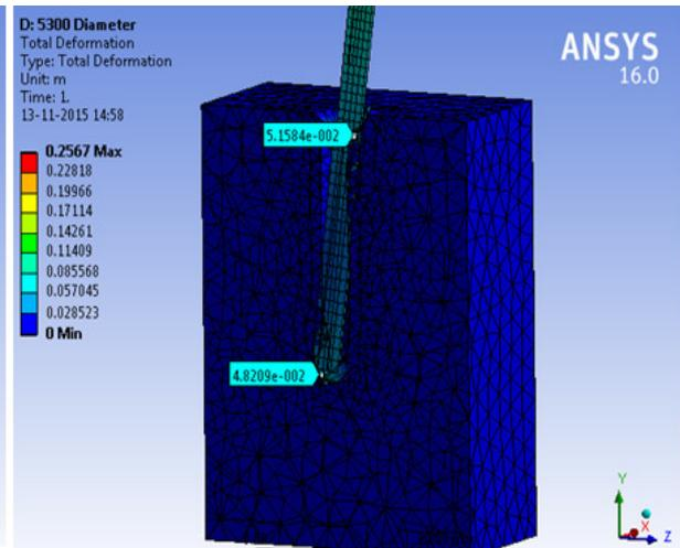
Fig. 9. Displacement at sea bed level of pile and pile toe of 5.3 m diameter pile.
