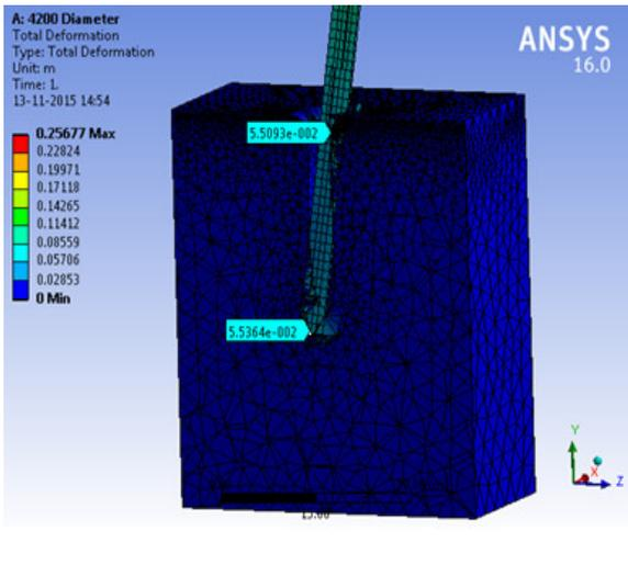
Fig. 6. Displacement at sea bed level of pile and pile toe of 4.2 m diameter pile.
