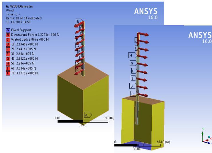
Fig. 5. Model of monopile, tower and soil in Ansys.
