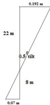
Fig. 4. Maximum displacement at 0.5° tilts at pile top and bottom.
