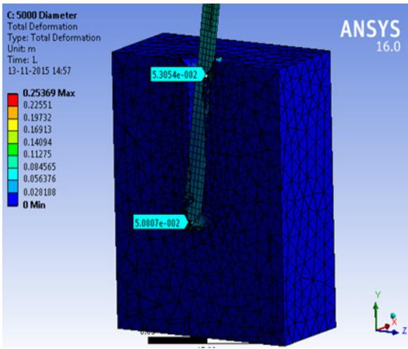
Fig. 8. Displacement at sea bed level of pile and pile toe of 5 m diameter pile.
