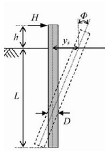
Fig. 3. Tilt of rigid monopile at pivot point.
