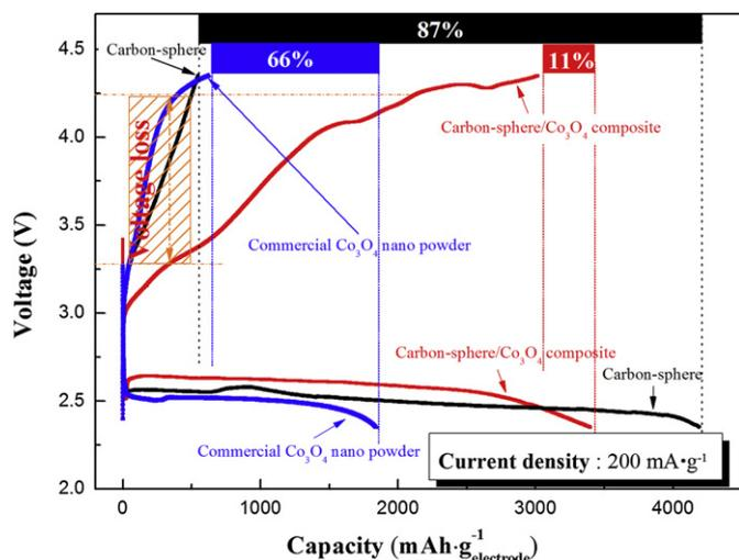
**Fig. 7.** Initial discharge/charge profiles of the air electrodes containing plain carbon spheres, commercial  $\text{Co}_3\text{O}_4$  nanopowder, and the carbon-sphere/ $\text{Co}_3\text{O}_4$  nanocomposite. The voltage range was 4.35–2.35 V and the current density was  $200 \text{ mA g}^{-1}$  (Top of the figure presents the difference between initial discharge capacity and charge capacity as %).
