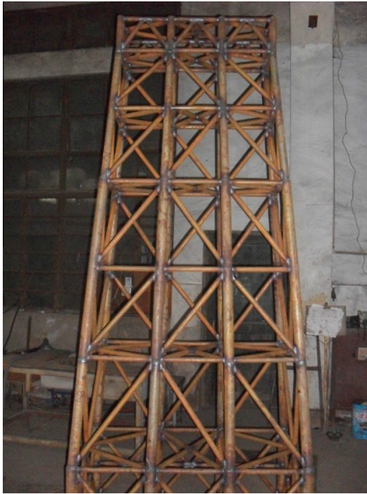
Fig. 5. The corrosion model of jacket.
