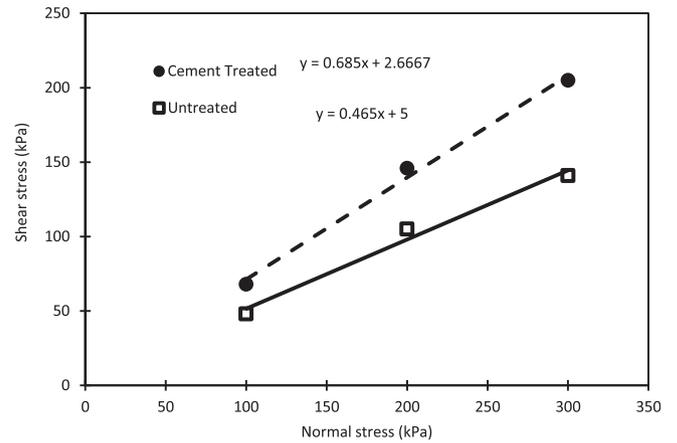
Fig. 3. Interface shear strength of sand and geotextile, and sand and cement-treated geotextile.
