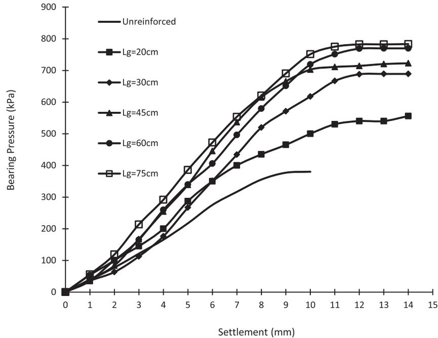
Fig. 6. Results of model tests on unreinforced and reinforced models with different reinforcement lengths.
