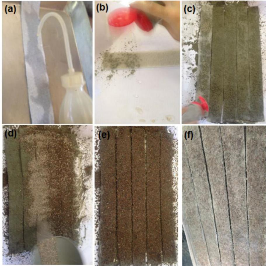
Fig. 1. Geotextile surface treated with cement and sand.
