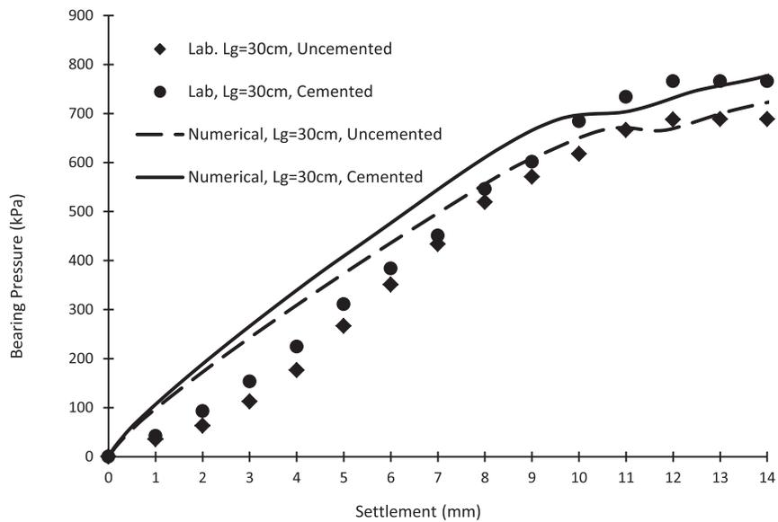
Fig. 15. Bearing capacity of reinforced model with and without cement-treated interface based on laboratory tests and numerical analysis (Lg = 30 cm).
