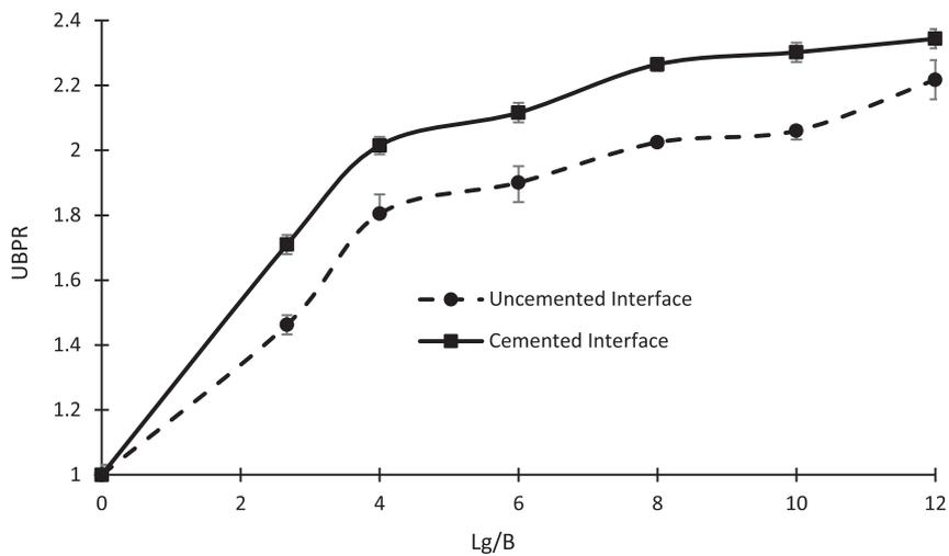
Fig. 10. Ratio of improvement in ultimate bearing capacity of reinforced models with and without cement-treated interfaces for 14 mm settlement.
