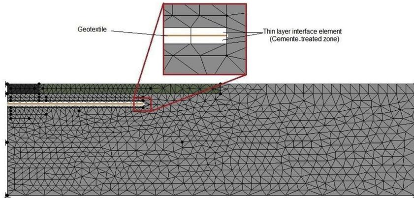
Fig. 13. Finite element model of the test setup.
