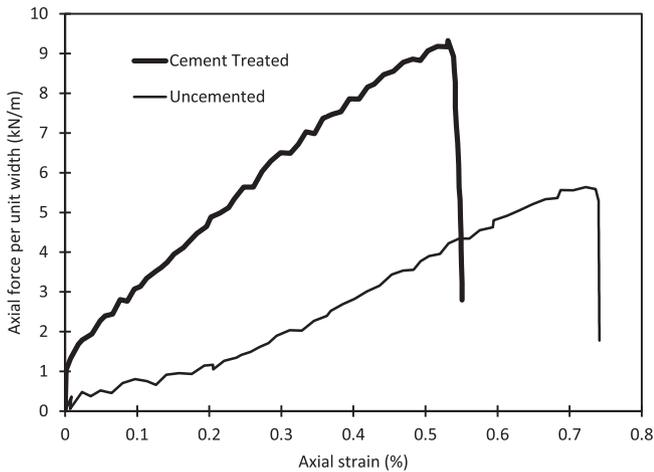
Fig. 2. Axial loading curves of cement-treated and pristine geotextiles.
