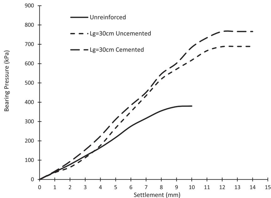
Fig. 7. Results of tests on unreinforced and reinforced models, and model reinforced with cement-treated interface with 30 cm reinforcement length.
