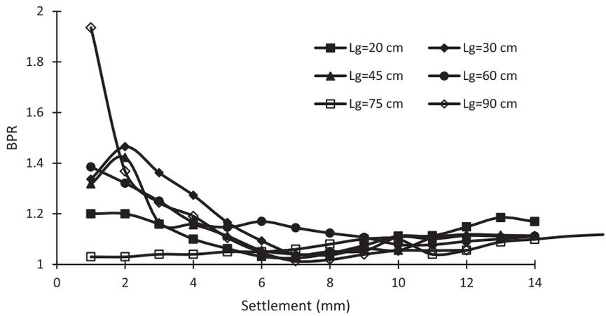
Fig. 9. Ratio of bearing pressure of reinforced models with cement-treated interfaces to the bearing pressure of reinforced models with pristine geotextile at different settlements.
