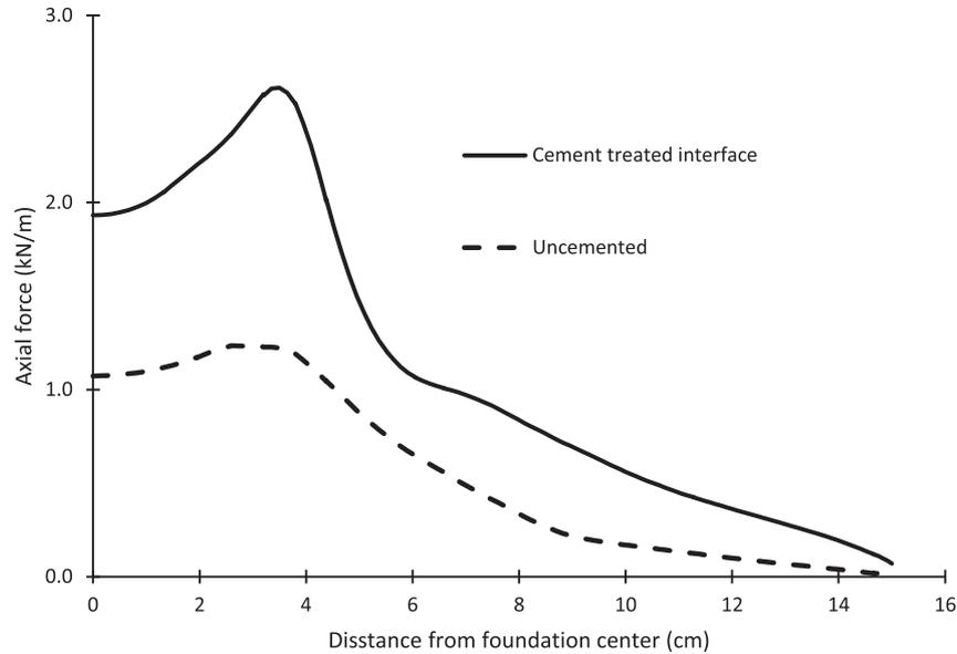
Fig. 16. Mobilized axial force of reinforcements ( $L_g = 30$  cm).
