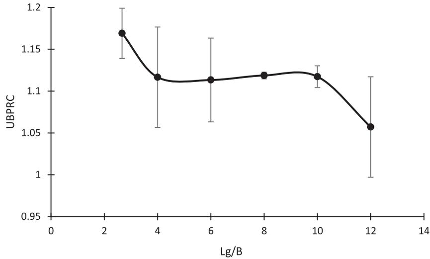
Fig. 11. Effect of cement-treated interface on the improvement of ultimate bearing capacity of reinforced soil.
