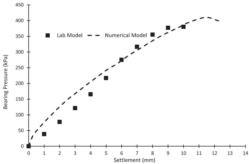
Fig. 14. Bearing capacity of unreinforced model based on laboratory testing and numerical analysis.
