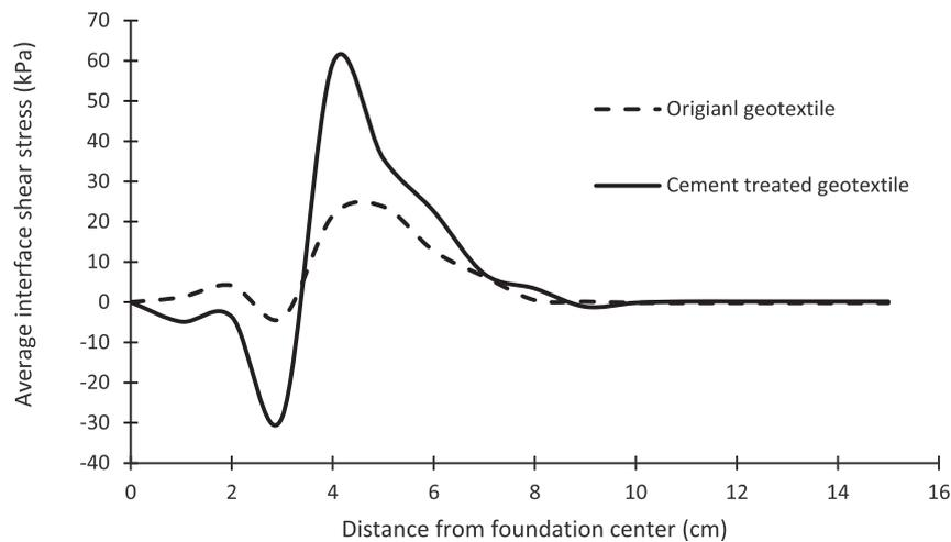
Fig. 17. Average mobilized interface shear stress ( $L_g = 30$  cm).
