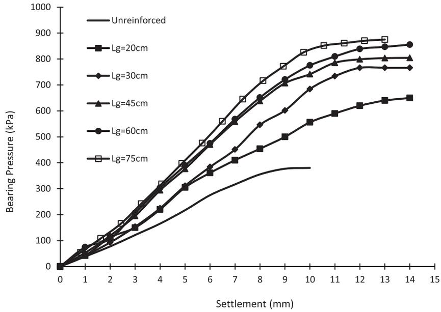
Fig. 8. Results of tests on unreinforced and reinforced models with cement-treated interface with different reinforcement lengths.
