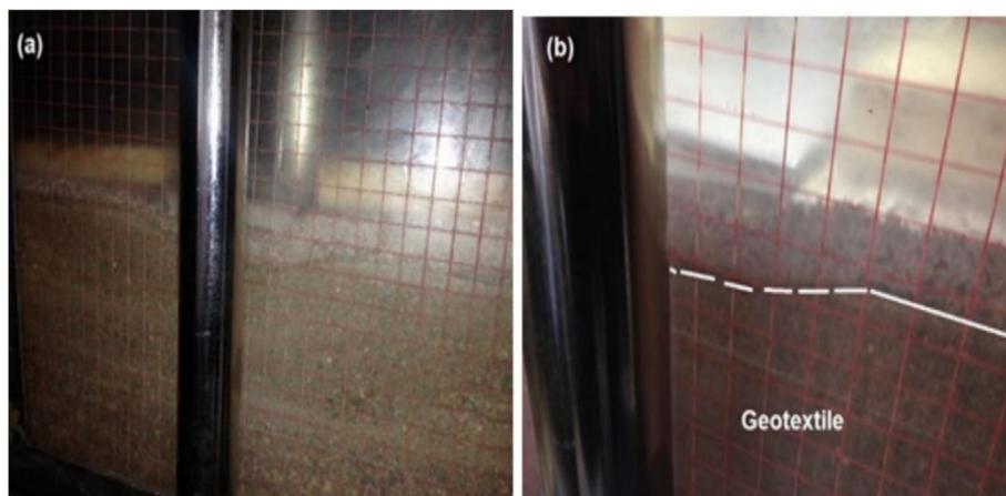
Fig. 5. Deformations of sand and geotextile layer after loading.
