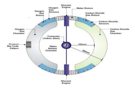
Figure 2. Internal cutaway view of respirocyte—equatorial view
