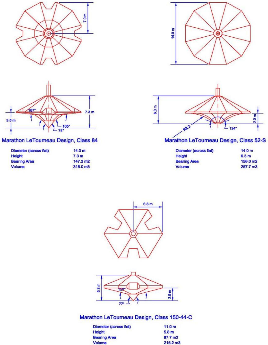
Fig. 2 (Cont.) Spudcan Geometries and Dimensions
