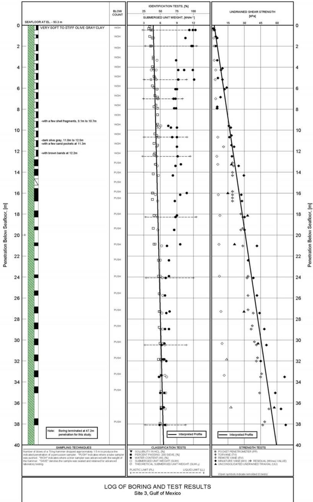
Fig. 1a Normally Consolidated Soil Profile for Site 3
