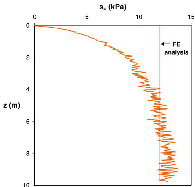
Figure 5 - Undrained shear strength profile of submerged OC clay
