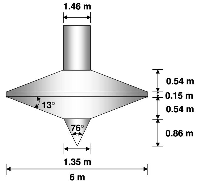
Figure 4 - Geometry of spudcan
