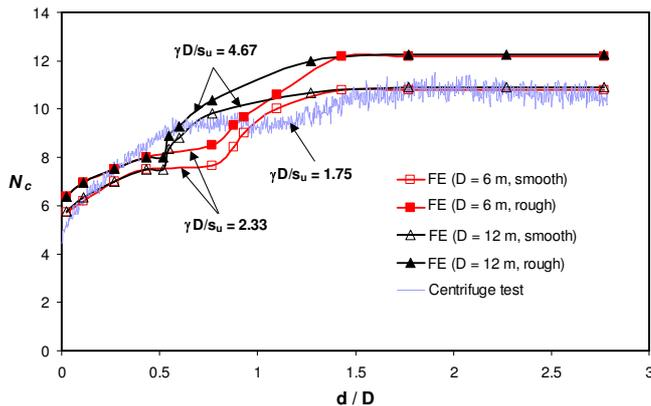
**Figure 9 - Bearing capacity factor,  $N_c$  of spudcan on uniform clay**
