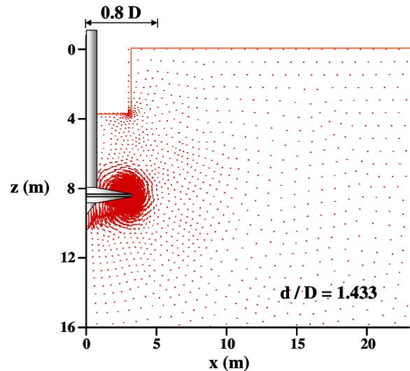
Figure 8 - Soil failure mechanisms from FE analysis
