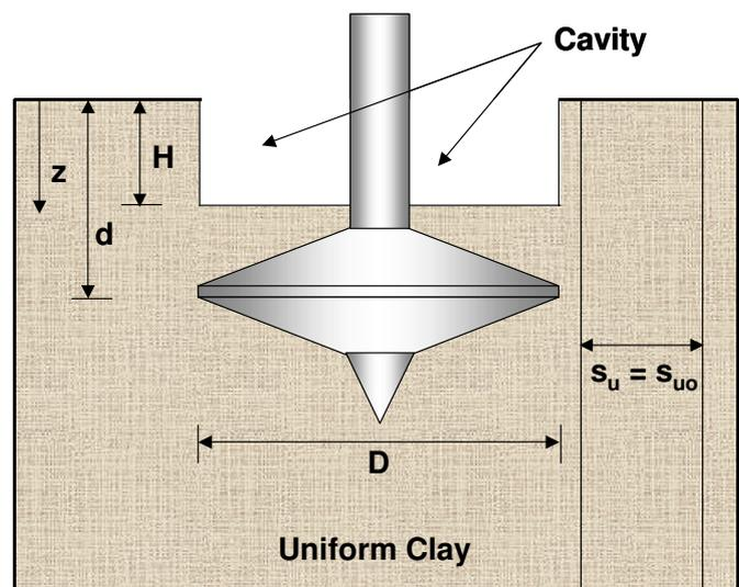
Figure 1 - Spudcan foundation in uniform clay
