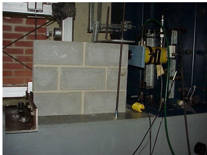
Figure 4. In-plane, destructive shear test set-up.
