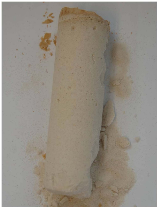
Fig. 3. Cemented sample after 3 days ( 100 \text{ kg/m}^3 )
