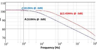
Fig. 3. CMRR~Frequency dependence Curve A refers to the circuit of Fig. 1. and B to the circuit of Fig. 2. Curve C refers to the circuit of Fig. 1. with increased I<sub>T</sub>
