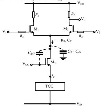
Fig. 1. Typical CMOS differential amplifier circuit  $R_T$ ,  $C_T$ ,  $C_{dg3}$ ,  $C_S$  and  $C_{db}$  are defined in the text
