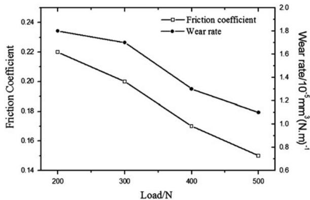
Figure 5. Effect of load on the friction coefficient and wear rate of CFRP composites (0.431 m/s).
