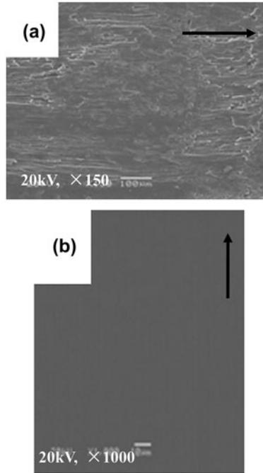
Figure 9. SEM images of the worn surface and transfer film of Gr/CNTs/CFRP composite at 500 N and 0.431 m/s. (a) worn surface; (b) transfer film of (a).
