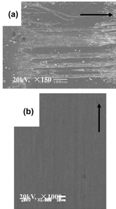
Figure 10. SEM images of the worn surface and transfer film of Gr/CNTs/CFRP composite at 200 N and 0.862 m/s. (a) worn surface. (b) transfer film of (a).
