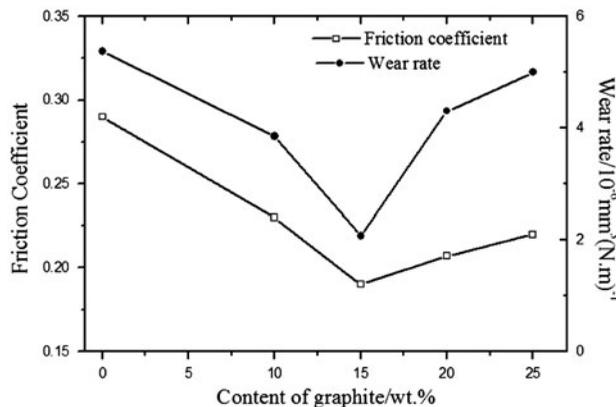
Figure 2. Friction coefficient and wear rate of Gr-filled CFRP composites (200 N, 0.431 m/s).
