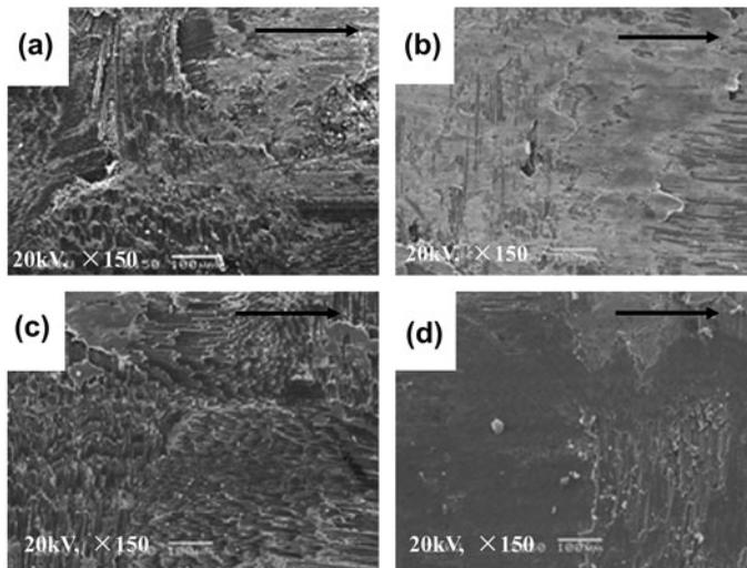
Figure 7. SEM images of the worn surface of the CFRP composites (200 N, 0.431 m/s) (a) Unfilled CFRP composites; (b) Gr/ CFRP composites; (c) CNTs/CFRP composites; (d) Gr/CNTs/CFRP composites.
