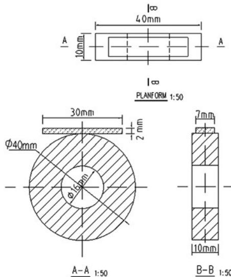
Figure 1. The contact schematic for the friction couple.
