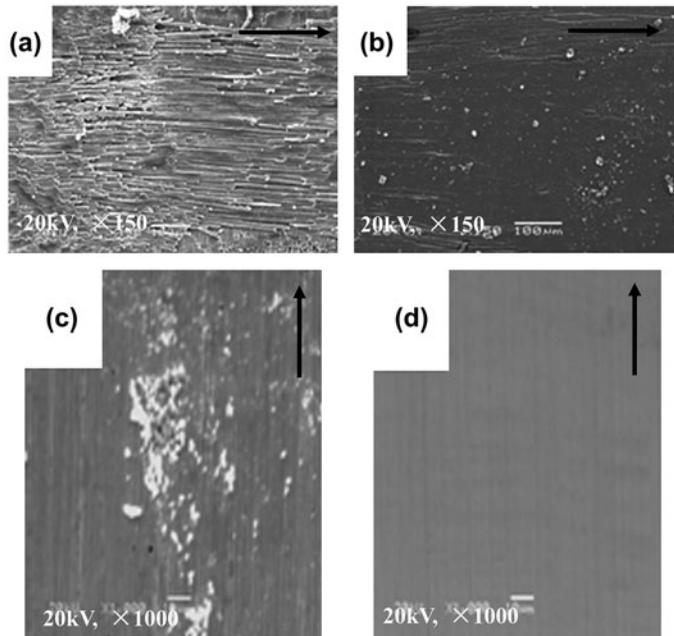
Figure 11. SEM images of the worn surface and transfer film of Gr/CNTs/CFRP composite under water and oil lubrication. (a) water lubrication; (b) oil lubrication; (c) transfer film of (a); (d) transfer film of (b).
