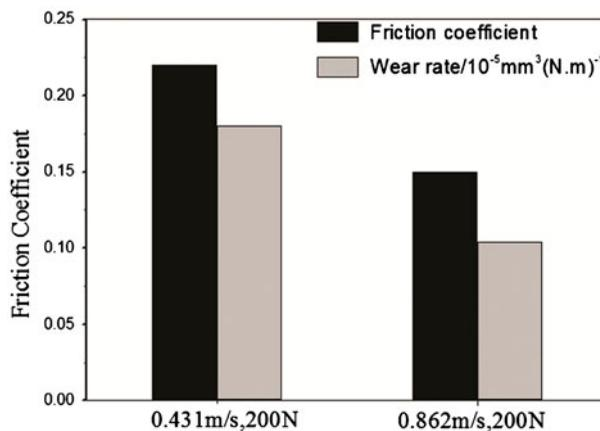
Figure 6. Effect of sliding speed on the friction coefficient and wear rate of CFRP composites (200 N).
