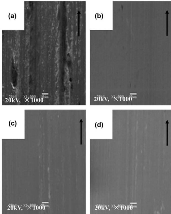
Figure 8. SEM images of the transfer film of the CFRP composites (200 N, 0.431 m/s). (a) Unfilled CFRP composites; (b) Gr/ CFRP composites; (c) CNTs/CFRP composites; (d) Gr/CNTs/CFRP composites.
