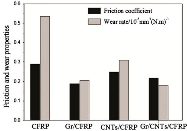
Figure 4. The combined effect of Gr and CNTs on the friction coefficient and wear rate of CFRP composites (200 N, 0.431 m/s).
