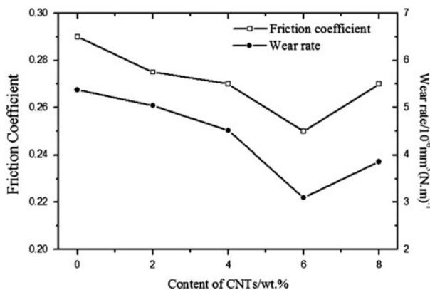
Figure 3. Friction coefficient and wear rate of CNTs-filled CFRP composites (200 N, 0.431 m/s).
