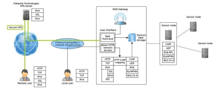
Fig. 3. System architecture of "Padova Smart City."
