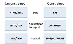
Fig. 2. Protocol stacks for unconstrained (left) and constrained (right) IoT nodes.
