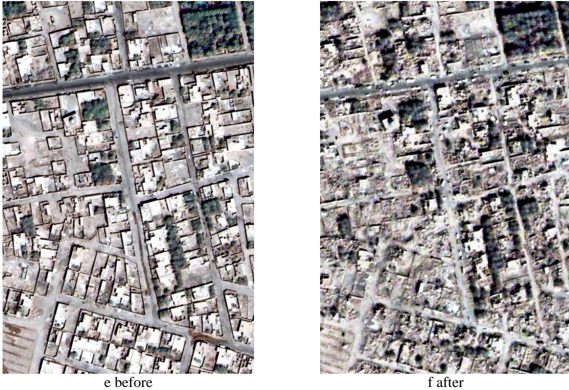
Figure 7 Building damage within eastern residential districts of Bam, visualized by comparing the ‘before’ and ‘after’ QuickBird satellite imagery. Imagery courtesy of DigitalGlobe, www.digitalglobe.com .
