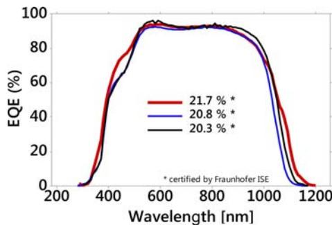
**Figure 1** External quantum efficiency (EQE) as measured and certified by Fraunhofer ISE of former (black and blue line) and current record cell (red thick line) (all with ARC).
