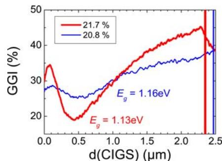
**Figure 2** Comparison of the GGI grading of the 21.7% (red thick line) and the 20.8% cell (blue thin line) as obtained from SNMS analysis. The vertical red and blue lines represent the end of the CIGS absorber and the transition to the molybdenum back contact.
