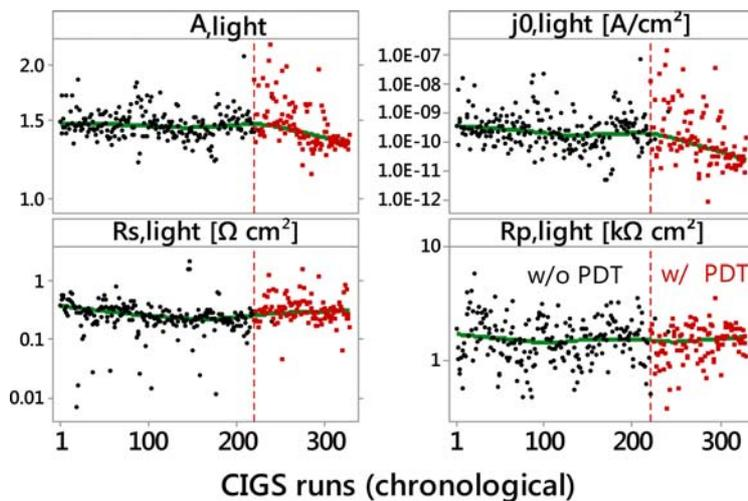
**Figure 3** Diode analysis (light  $I$ - $V$  curves) of chronological ZSW small area cell production over the past years (only best solar cell of each production run depicted). For CIGS solar cells with PDT (red squares) a trend towards smaller diode quality factors  $A$  and saturation current densities  $J_0$  can be observed.
