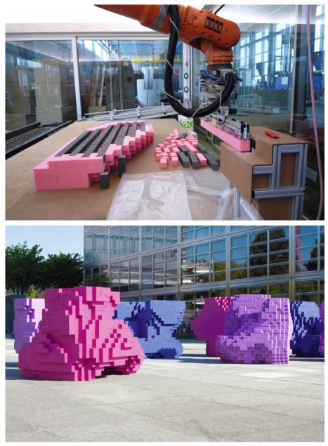
Fig. 5. a, above) Foam blocks of different density and hardness are distributed over the cross section in order to control localized performance properties; b, below) The finished furniture pieces are coated with a layer of Polyurethane
