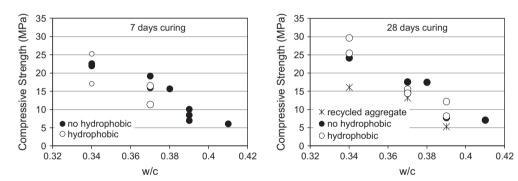
Fig. 4. Compressive strength as a function of w/c for different mixtures after 7 days and 28 days of curing.
