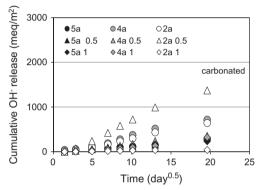
Fig. 11. Release of hydroxyl ions by no-fines concretes before (left) and after (right) carbonation. In the left graph, the black line shows the release trend of an ordinary concrete as reference (CEM II/A-L 42.5 R w/c = 0.6).
