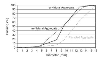
**Fig. 1.** Particle size distribution of natural and recycled aggregate from different lab ("m" = Milan; "a" = Ancona).
