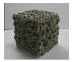
Fig. 3. No-fines concrete specimen.
