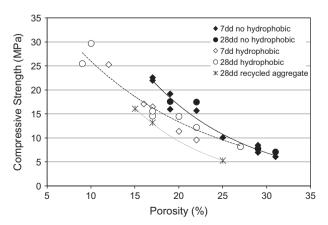
**Fig. 5.** Compressive strength after 7 and 28 days of curing as a function of porosity for different mixtures.
