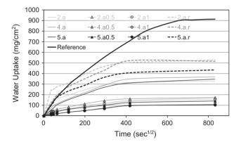
Fig. 9. Capillary water absorbed by no-fines concretes.
