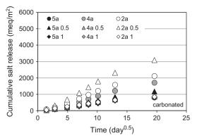
Fig. 10. Release of salt constituent by no-fines concretes before (left) and after (right) carbonation. In the left graph, the black line shows the release trend of an ordinary concrete as reference (CEM II/A-L 42.5 R w/c = 0.6).
