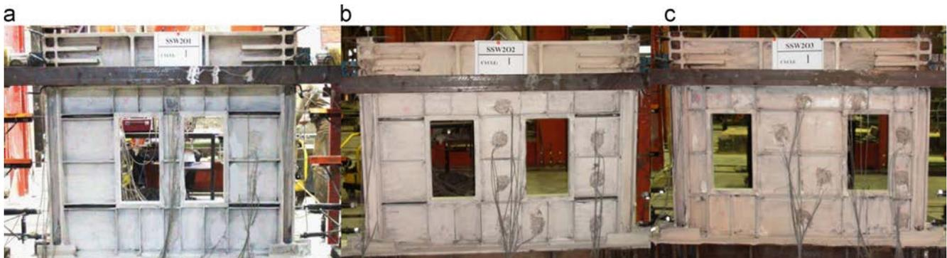
Fig. 4. Experimental specimens before conducting the test. (a) SSW201, (b) SSW202, and (c) SSW203.
