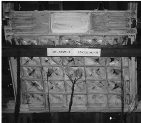
Fig. 10. Deformation of DS-SPSW-0% specimen at 6.44% drift.
