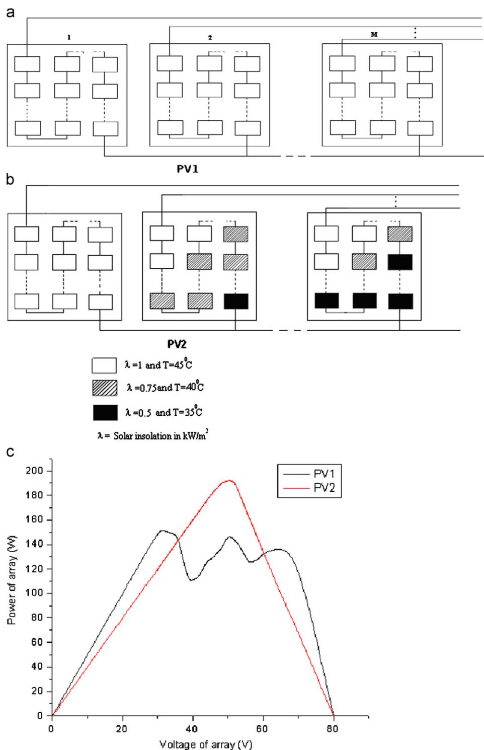
**Fig. 1.** (a) PV array configuration of module PV1 (under total illumination). (b) PV array configuration of module PV2 (under partial shading). (c) Power – vs. – voltage characteristics of modules PV1 and PV2.
