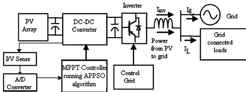
Fig. 5. System configuration for grid connected PV-based system.
