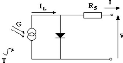
Fig. 4. Circuit model of a PV cell.
