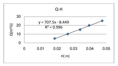
Fig. 6: Relation of scale flow rate for spillway with flat bed.
