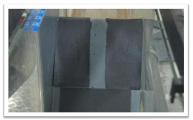
Fig. 4: How to create roughness on spillway surface.
