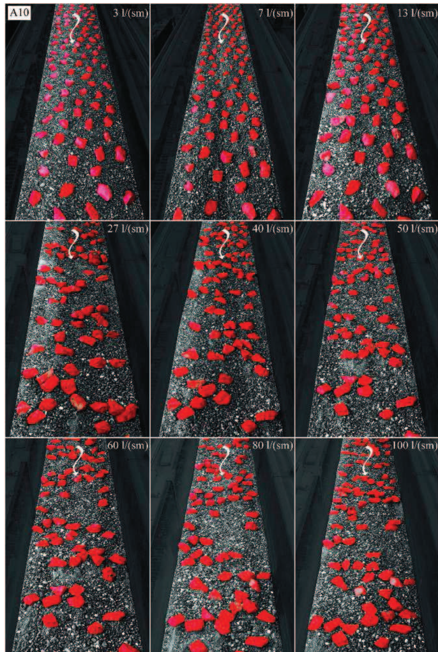
Fig. 6. Experiment A10 (Table 2) taken after different runs, showing the partial movement of the blocks forming more structured pattern during large discharges
