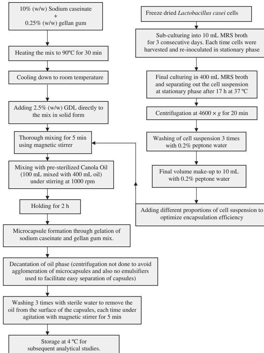
Fig. 1. Optimized process flow diagram of the cell culturing and microencapsulation of *Lactobacillus casei* 431 bacteria.
