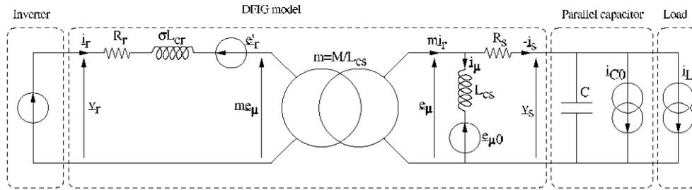
Figure 5: Global dynamical equivalent circuit in a grid synchronous frame
