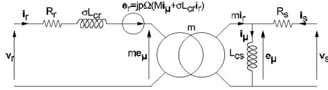
Figure 2: Equivalent circuit of the DFIG
