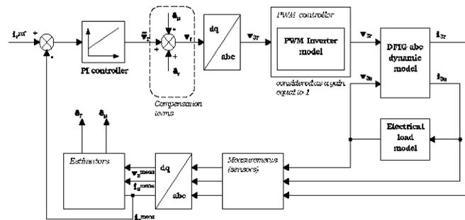
Figure 6: Inner rotor current loop
