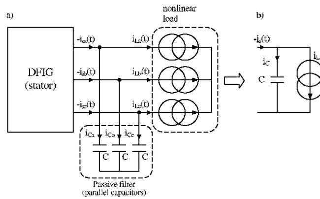
Figure 3: Three-phase nonlinear load with parallel capacitors (a) and its dynamical equivalent circuit (b)
