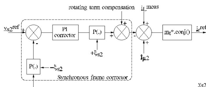
Figure 8: Stator voltage controller
