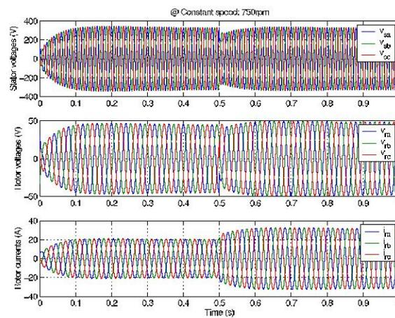
Figure 11: DFIG behaviour with a variation of load
