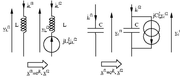
Figure 4: Transformation by rotation of reactive components (from f1 reference frame to f2 reference frame)
