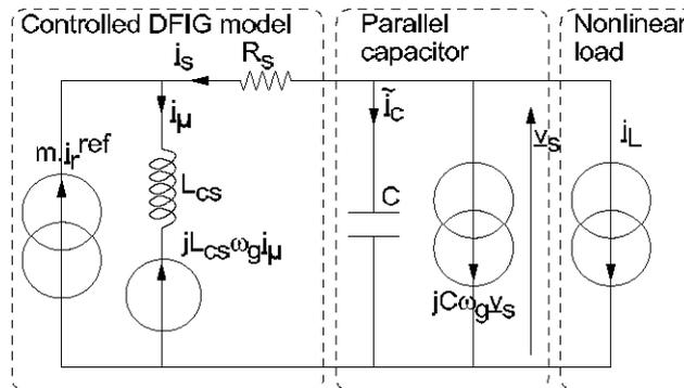
Figure 7: Controlled DFIG model
