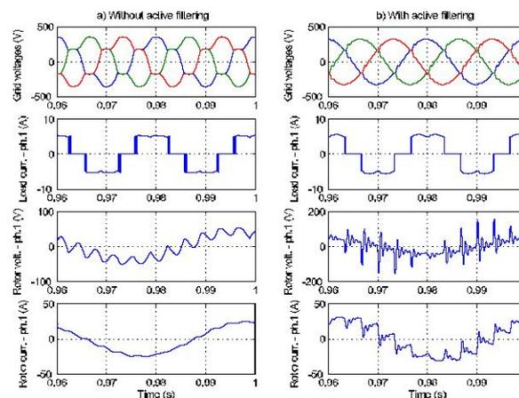
Figure 13: Active filtering operation (a - without and b - with active filtering)
