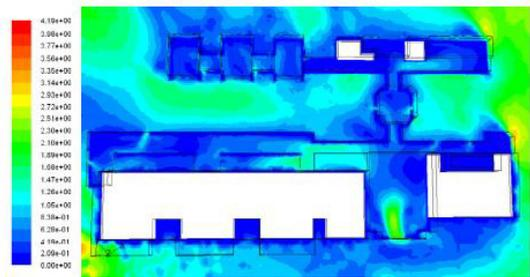
Fig. 12. wind speed levels at level 1.5m in rooms on F1 after preliminary adjustment.
