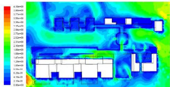
Fig. 14. wind speed levels at level 1.5m in rooms on F1 after final optimization.
