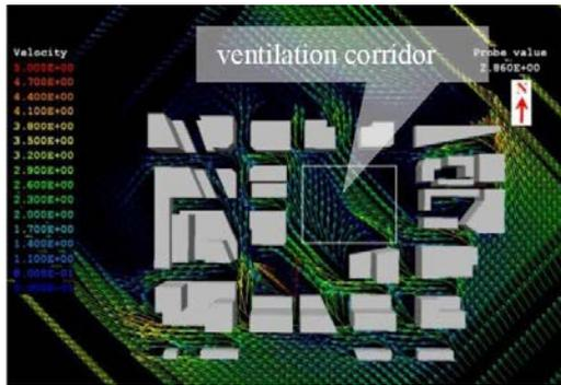
Fig. 1. vector of wind speed distribution at pedestrian height on the site.
