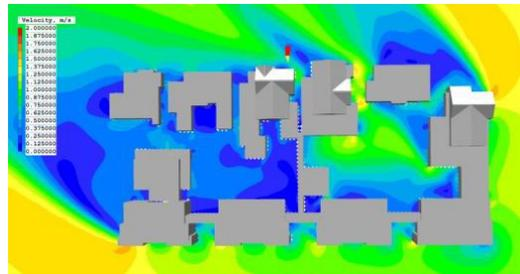
Fig. 4. wind speed levels – all corridors enclosed.
