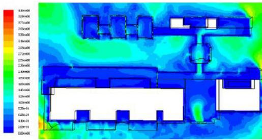
Fig. 11. wind speed levels at level 1.5m in rooms on F1 in preliminary simulation.
