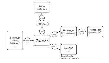
► Figure 6. Overview of the digital chain with standard software solutions.
