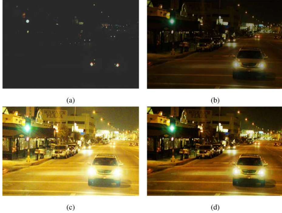
Fig. 4. (a) Original image before Gamma correction. (b) After Gamma correction. (c) Gamma correction followed by histogram equalization. (d) Joint Gamma correction and contrast-tone optimization by the proposed OCTM method.
