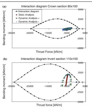
**Fig. 12** Interaction diagram (*solid line with squares*) of the transversal cross-section of the Serro Montefalco tunnel at crown (**a**) and at invert (**b**), adding the dynamic stress increment as both a positive (*squares*) and negative (*triangles*) contributions to the static contribution (*circles*)
