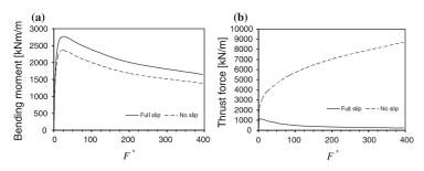
Fig. 10 Effect of the contact condition at the rock-mass-lining interfaces (full slip (*solid line*) and no slip (*dashed line*)) on the increment of the internal forces on the lining under seismic loading versus the flexibility ratio F\*: a bending moment; b thrust force
