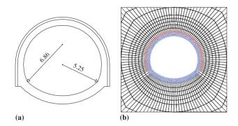
Fig. 4 a Cross-section of the "Serro Montefalco" tunnel; b mesh of the FLAC model
