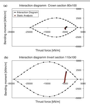
Fig. 6 Interaction diagrams (*solid line with squares*) for the tunnel cross-section in static condition (*circles*): a crown section  $80 \times 100$ ; b invert section  $110 \times 100$
