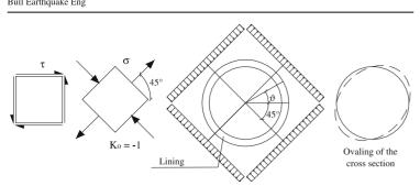
Fig. 8 State of stress around a tunnel corresponding to uniform, pure shear deformation
