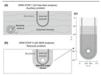
Fig. 7 DRM procedure applied to the case study. **a** Step I: free-field analysis of the wave propagation from the seismic source; **b** Step II: wave propagation in the reduced domain including soil-structure interaction. The *dark line* denotes the effective boundary. **c** SE model of the reduced problem including the transversal A–A' cross-section of the tunnel
