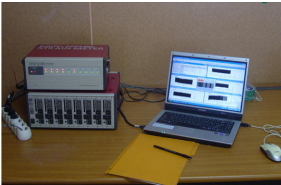
Fig. 3. The digital dynamic strain meter, the amplifier, and the computer.
