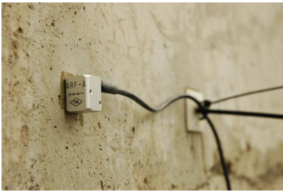
Fig. 2. Accelerometers (Tokyo-Sokki ARF-A) mounted on the outer surface of the containment.
