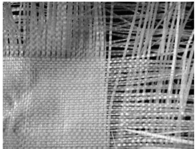
Fig. 4. Fiber bundles split from waste polymer textile bags.
