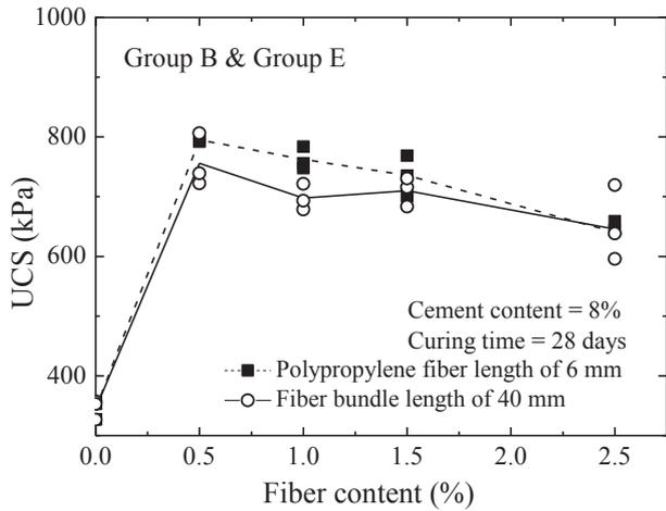
Fig. 11. UCS of the improved clay versus fiber contents.
