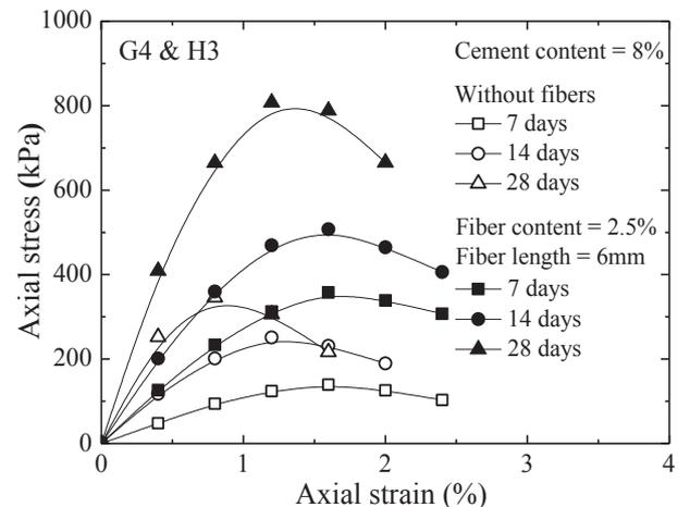
Fig. 14. Stress–strain curves for without-fiber specimens and polypropylene fiber-reinforced specimens with different curing time.
