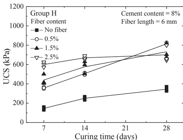
Fig. 16. Effect of curing time for specimens with different polypropylene contents.
