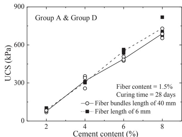
Fig. 10. UCS of the improved clay versus cement contents.
