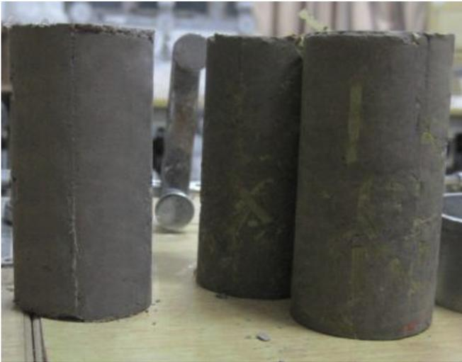
Fig. 5. Fiber-reinforced cement–clay specimens.
