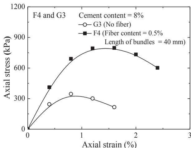
Fig. 9. Stress–strain curves for specimens without & with fiber bundles.
