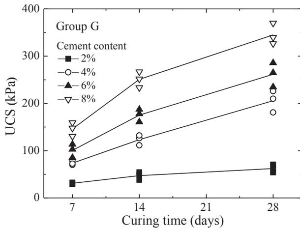
Fig. 15. Effect of curing time for specimens without fiber.
