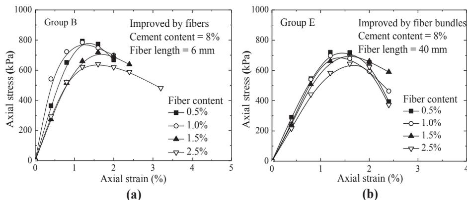
Fig. 7. Stress–strain curves for specimens improved with different fiber content under cement content 8%: a) fibers and b) fiber bundles.
