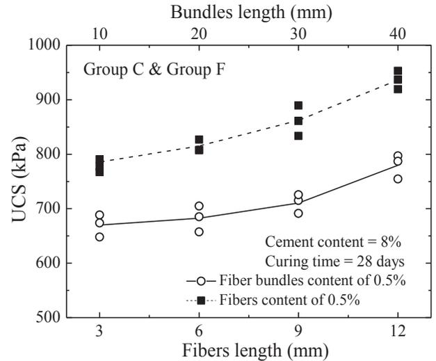
Fig. 13. UCS of the improved clay versus fiber lengths.
