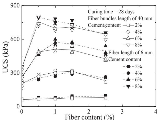
Fig. 12. UCS of the improved clay with different cement contents versus fiber contents.
