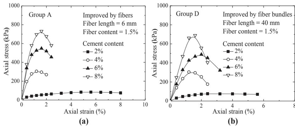
Fig. 6. Stress–strain curves for specimens improved with different cement content under fiber content 1.5%: a) fibers and b) fiber bundles.
