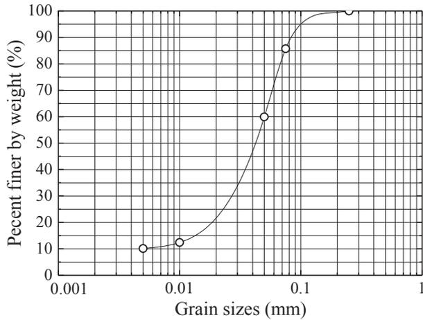
Fig. 2. Grain distribution size curve for Shanghai clay used in the tests.
