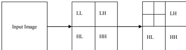
**Figure 2.** Flow chart of the DWT sub band coding
