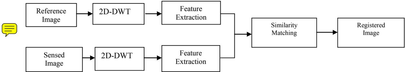
**Figure 1.** Block Diagram of Image Registration
