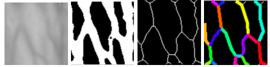
Figure 3. LEM extraction steps: A vein image, Yasuda binarization and noise removal, skeletonization and line segments generation
