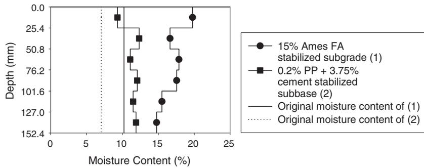
Fig. 4. Moisture content profiles of two different specimens.
