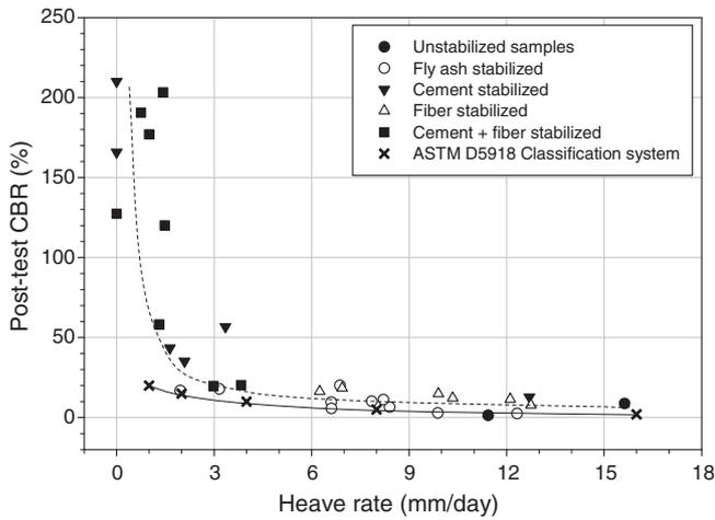
Fig. 10. Relationships between Post-test CBR and measured heave rates with comparison to the ASTM D5918 criteria.
