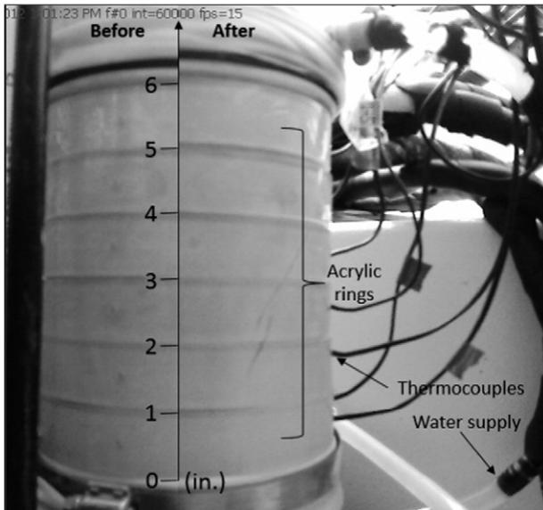
Fig. 2. Side by side specimen assembly before/after freeze-thaw testing (1 in. = 25.4 mm).
