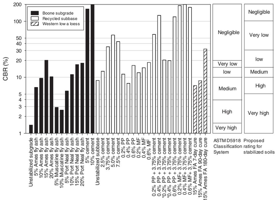
Fig. 9. Post-test CBR values and corresponding frost susceptibility ratings based on ASTM and the results from this study.
