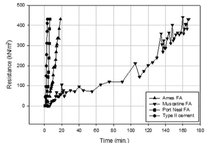
**Fig. 6.** Penetration resistance set time plots for fly ash and cement.
