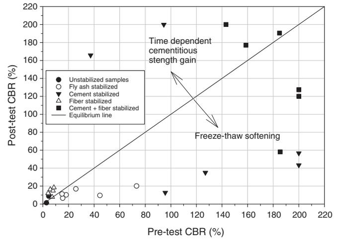
Fig. 11. Comparison between pre and post-test CBR values showing the influence of time dependent strength gain for cement and cement + fiber stabilized specimens.
