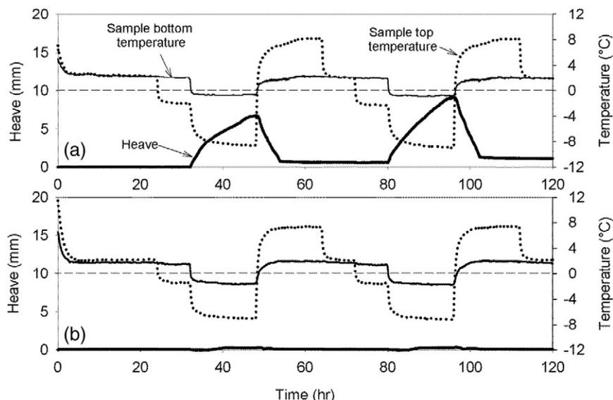
Fig. 5. Frost-heave time plots of (a) 0.2% PP fiber stabilized subbase and (b) 10% cement stabilized subgrade.
