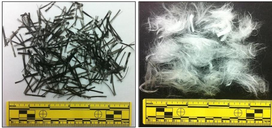
Fig. 7. White monofilament fibers (MF) (left) and black polypropylene fibers (PP) (right).
