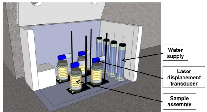
Fig. 3. Idealized view of the temperature control chamber (Johnson, 2012).
