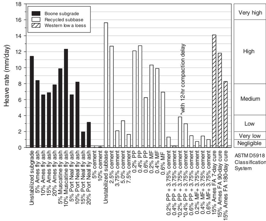
Fig. 8. Comparison of frost-heave rates of all tested materials.
