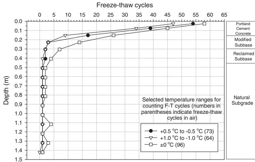
Fig. 1. Freeze-thaw profile of a typical Iowa pavement foundation (data collected in Boone County, IA Hwy 30, from Fall 2013 through Spring 2014).
