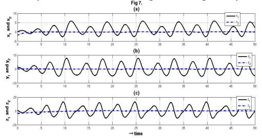
Fig.7. Solution of Genesio system and NSG systems with the active control deactivated.
