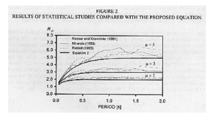
Miranda (1996) has shown that the use of approximate reduction Pictors like those computed with equation 2 combined with the use of smoothed linear elastic response spectra (SLERS) can lead to very good estimates inelastic strength demands (i.e., lateral strength required to control displacement ductility demands).
